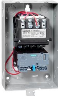
Non-reversing motor starter Size 00 Three phase full voltage Solid-state overload relay OLRelay amp range 3-12A 208VAC 60HZ coil Combination type Indoor general purpose use
