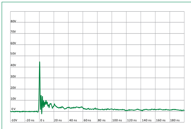
IEC 61000-4-2 +8 kV Contact ESD Clamping Voltage
