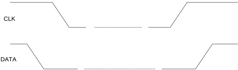
Figure 18: Timing of START and STOP Condition
