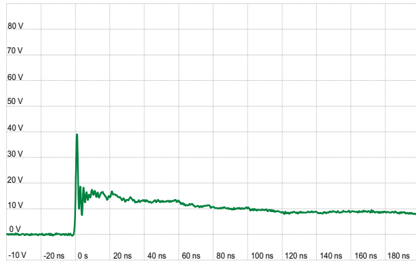
IEC 61000-4-2 +8 kV Contact ESD Clamping Voltage
