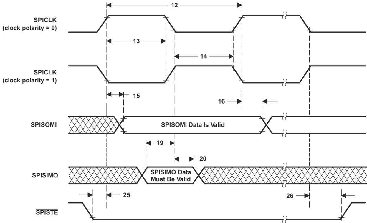
Figure 6-72. SPI Slave Mode External Timing (Clock Phase = 0)
