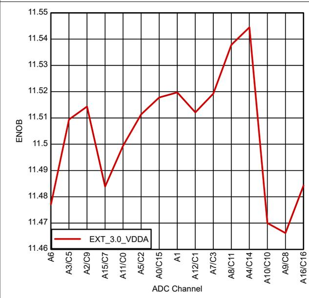
**Figure 6-44. Per-Channel ENOB for 32-Pin RHB VQFN**
