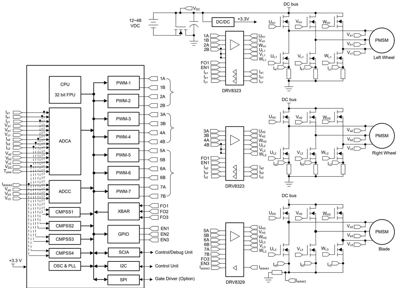
**Figure 8-8. Single-Chip Solution for Robotic Lawn Mower**
