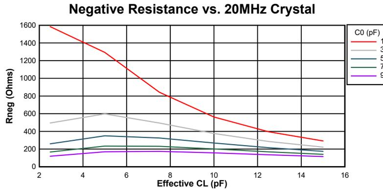
**Figure 6-20. Negative Resistance Variation at 20 MHz**
