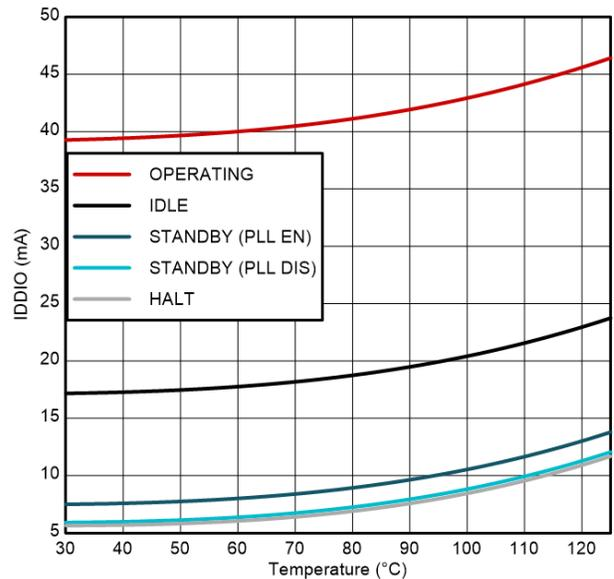
**Figure 6-2. Current Versus Temperature - Internal Supply**
