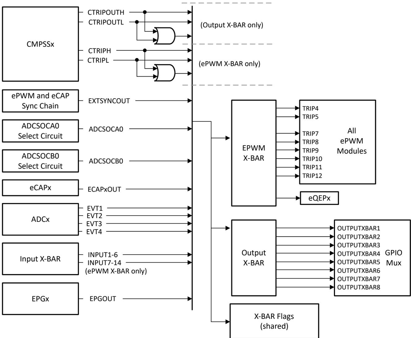
Figure 5-7. Output X-BAR and ePWM X-BAR Sources
