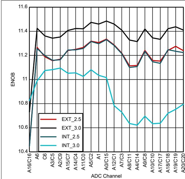
**Figure 6-41. Per-Channel ENOB for 64-Pin PM LQFP**
