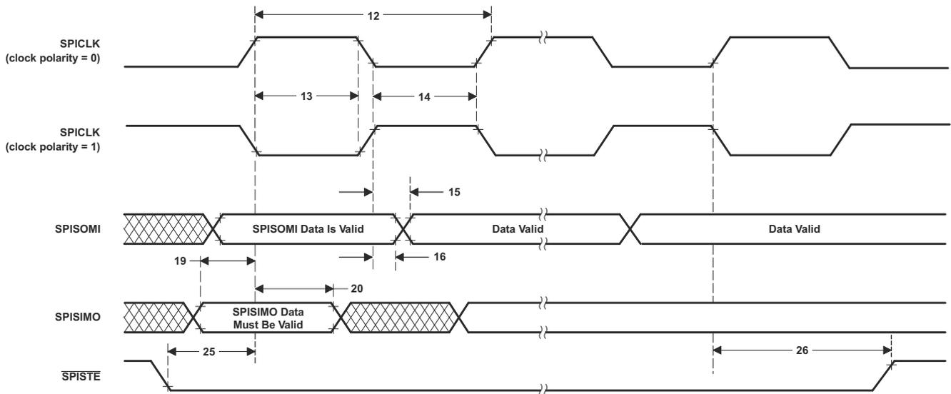
Figure 6-73. SPI Slave Mode External Timing (Clock Phase = 1)
