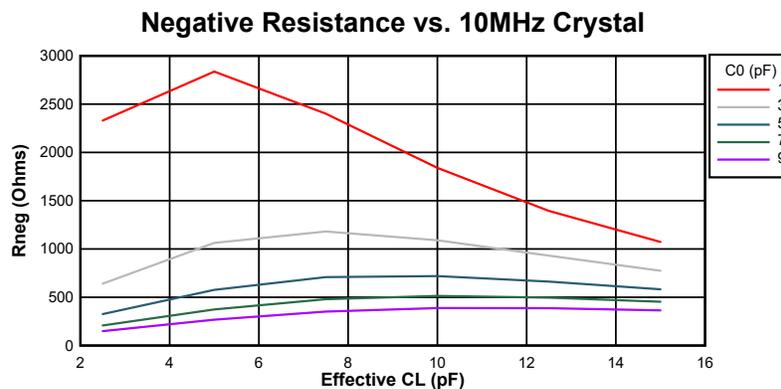
**Figure 6-19. Negative Resistance Variation at 10 MHz**
