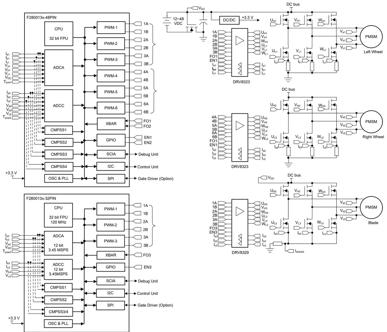
**Figure 8-7. Dual-Chip Solution for Robotic Lawn Mower**
