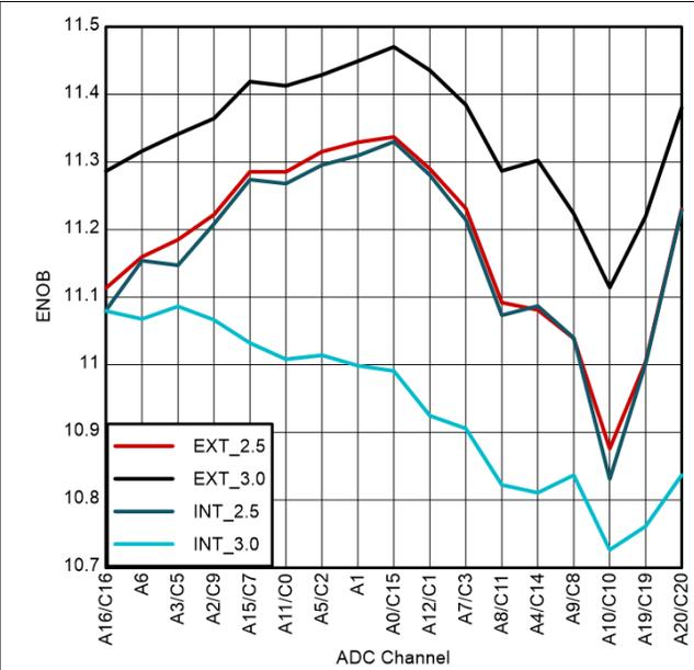
**Figure 6-42. Per-Channel ENOB for 48-Pin PT LQFP**
