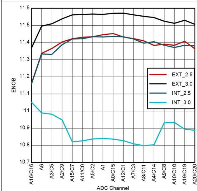
**Figure 6-43. Per-Channel ENOB for 48-Pin RGZ VQFN**
