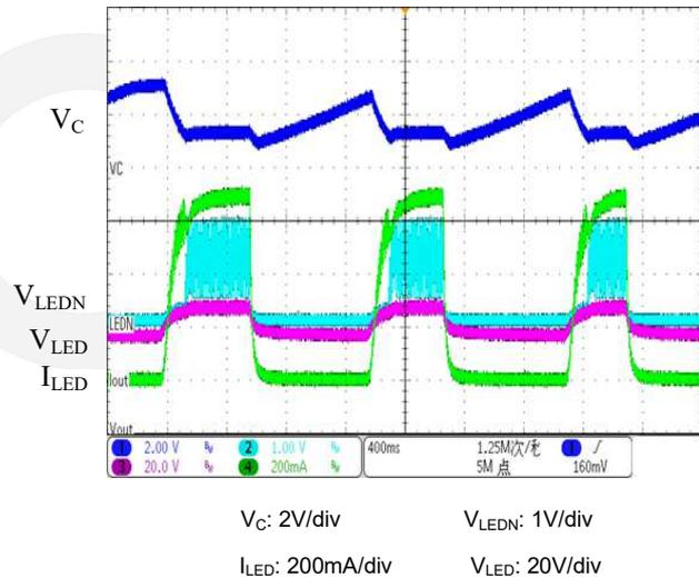
Fast dimming application test
