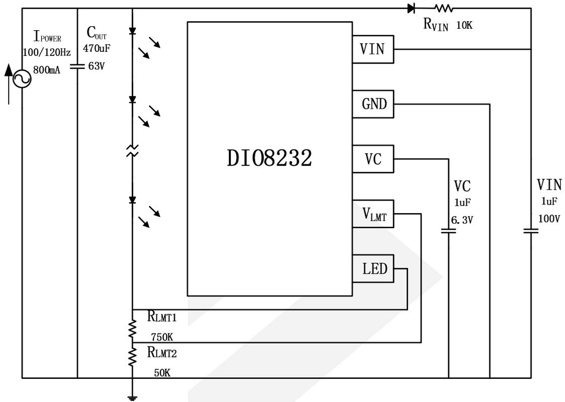
Adaptive 100/120Hz Current Ripple Remover, Max Input Current  $\leq 1A$
