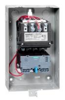
Non-reversing motor starter, Size 0, Three phase full voltage, Solid-state overload relay, OLRelay amp range 0.25-1a, 220 240/440 480VAC 60HZ coil, Non-combination type, Enclosure type 12, Dust/drip proof for indoors, Standard width enclosure
