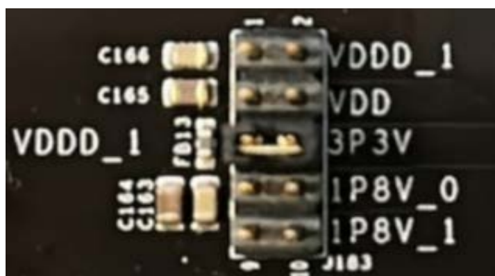
Figure 6. Power Source Selector for V_{DDD} _1
