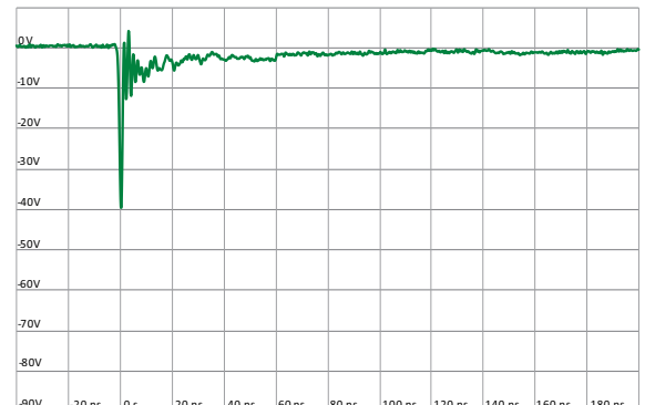
IEC 61000-4-2 -8 kV Contact ESD Clamping Voltage
