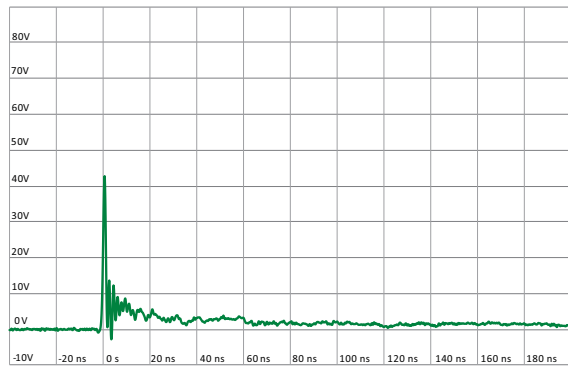
IEC 61000-4-2 +8 kV Contact ESD Clamping Voltage
