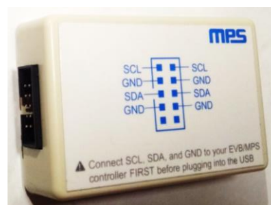
Figure 3: EVKT-USBI2C-02 Communication Interface
