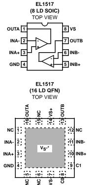
\*THERMAL PAD MUST BE CONNECTED TO NEGATIVE SUPPLY:  $\rm V_{S^{-}}$  QFN PACKAGE CAN BE USED IN DUAL SUPPLY APPLICATIONS.
