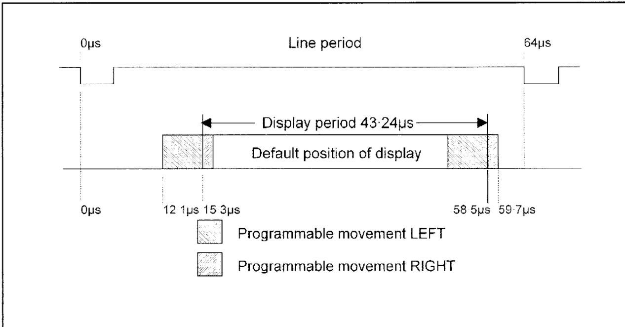
Fig. 10 Horizontal position and movement of text display.
