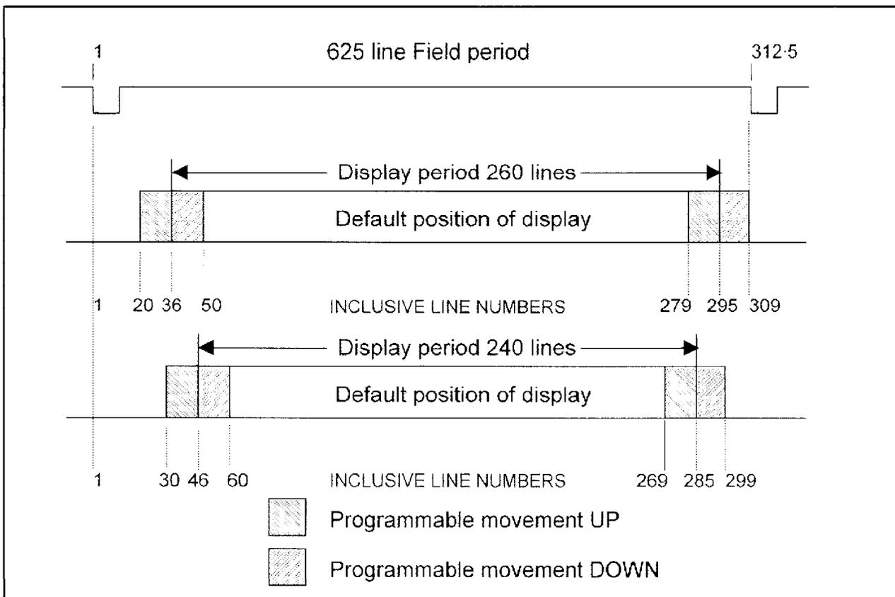
Fig. 11 Vertical position and movement of text display.
