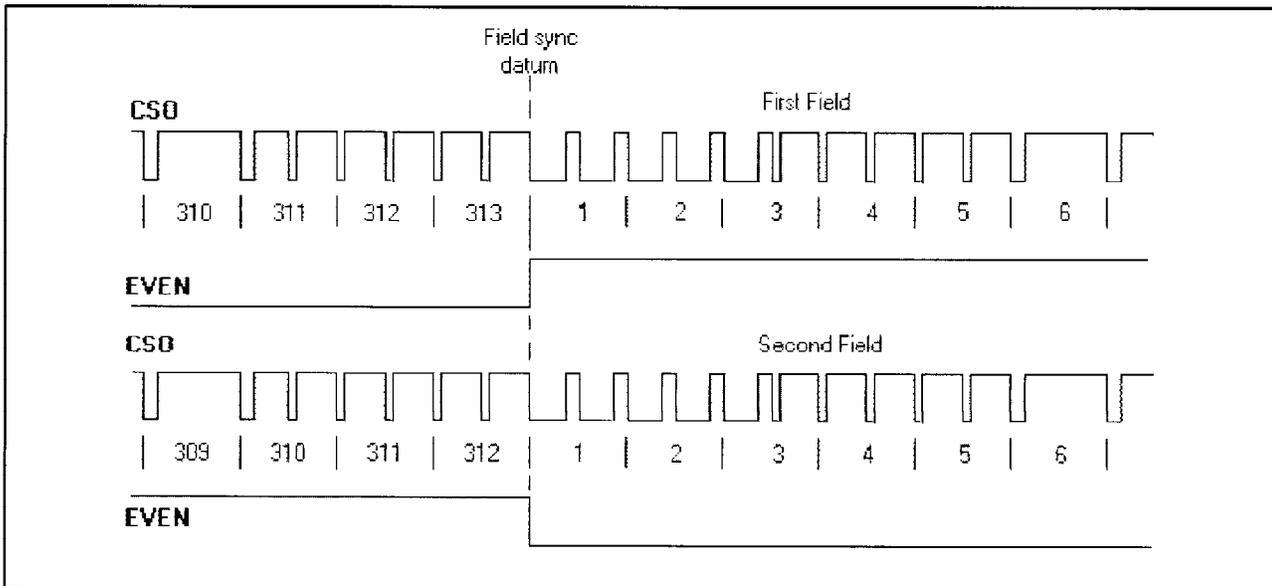
Fig. 6b. Composite sync output (non-interlaced 312:313) and EVEN output.
