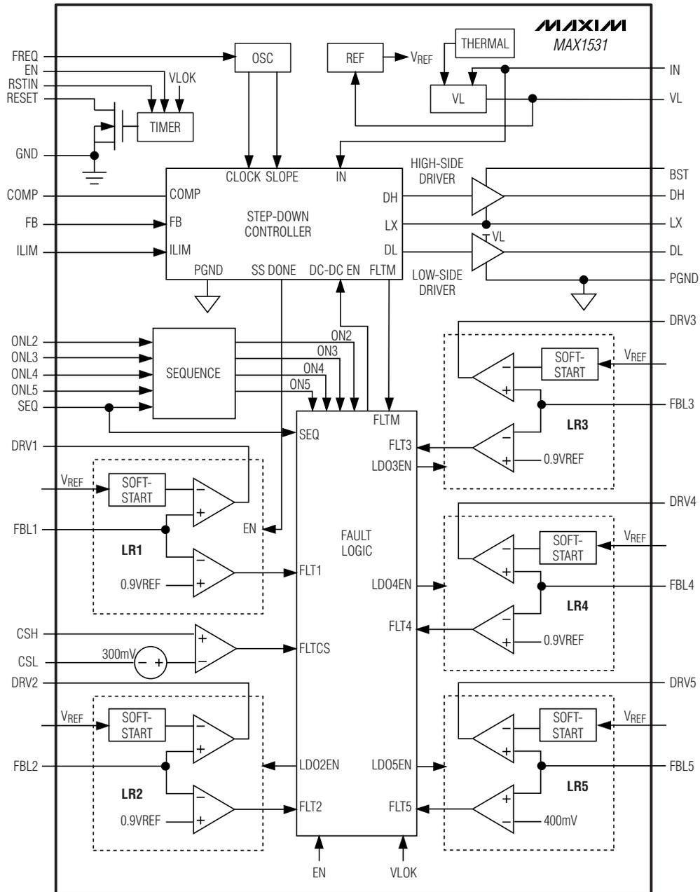
Figure 3. IC Functional Diagram
