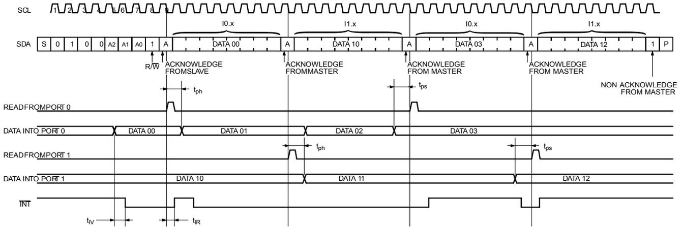
**Note:** Transfer of data can be stopped at any moment by a STOP condition. When this occurs, data present at the latest acknowledge phase is valid (output mode). It is assumed that the command byte has previously been set to 00 (read input port register).
