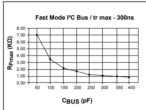
Figure 3. Maximum  $R_P$  Value versus Bus Capacitance
