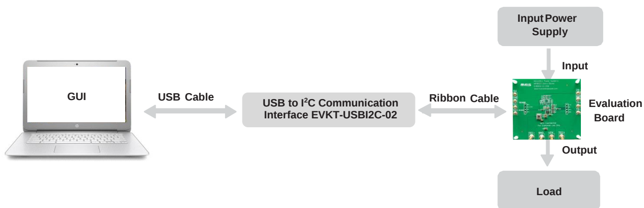
Figure 1: EVKT-MP8833 Evaluation Kit Set-Up
