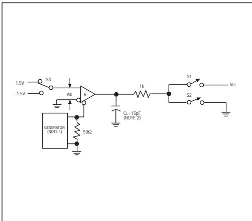
Figure 7. Receiver Enable and Disable Timing Circuit
