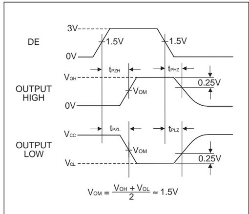
Figure 10. Driver Enable and Disable Timing Waveforms
