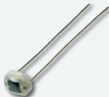
Planar silicon photodiode mounted on a ceramic substrate and coated with a layer of clear epoxy
