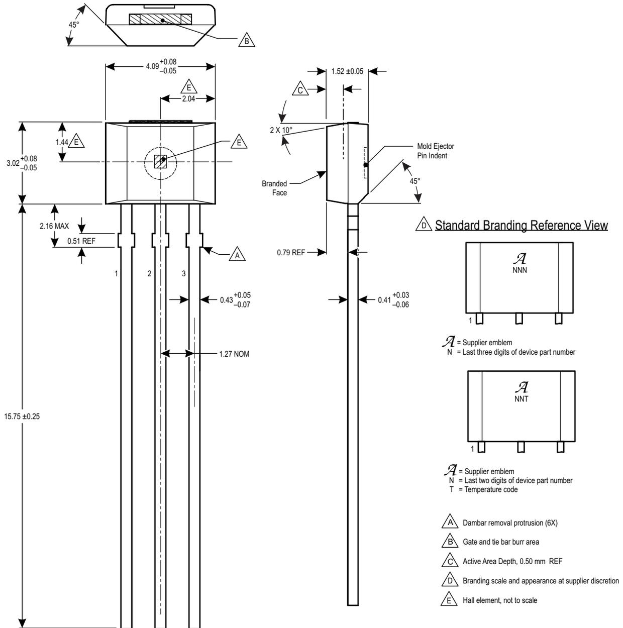
**Figure 4: Package UA, 3-Pin SIP, Matrix Style**
