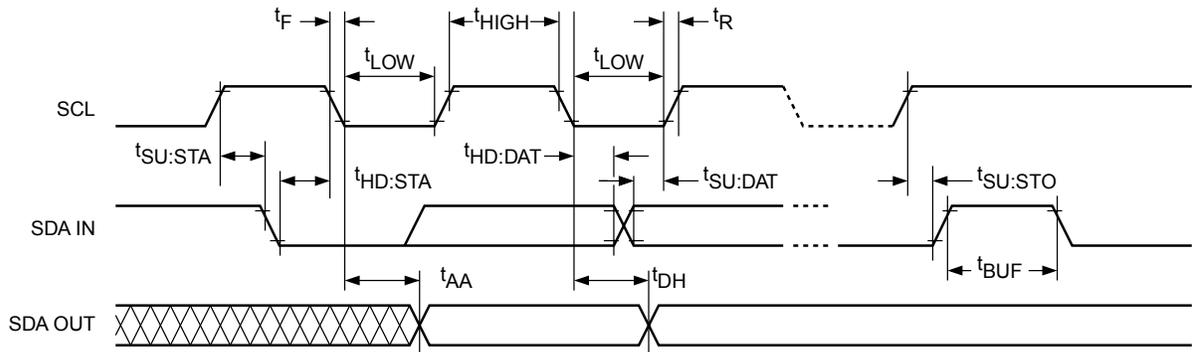
**Figure 1. 2-Wire Serial Interface Timing**
