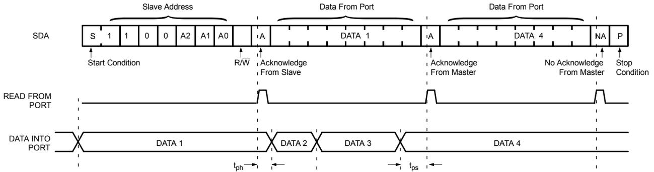
**Figure 8. Read Input Port Register Timing Diagram**
