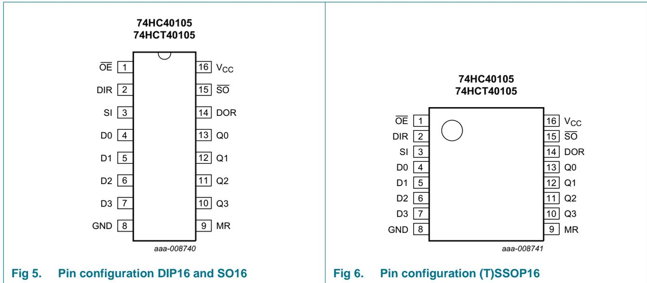
Fig 5. Pin configuration DIP16 and SO16
