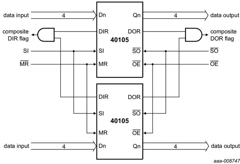
The 74HC40105; 74HCT40105 is easily expanded to increase word length. Composite DIR and DOR flags are formed with the addition of an AND gate. The basic operation and timing are identical to a single FIFO, except for an added gate delay on the flags.
