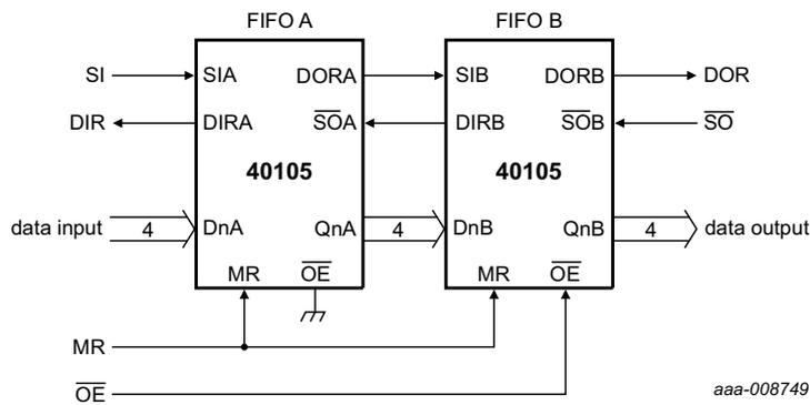
The 74HC40105; 74HCT40105 is easily cascaded to increase word capacity without external circuitry. In cascaded format, the FIFOs handle all necessary communications. Figure 19 and Figure 21 demonstrate the communication timing between FIFOA and FIFOB. Figure 24 provides an overview of pulses and timing of two cascaded FIFOs, when shifted full and shifted empty again.
