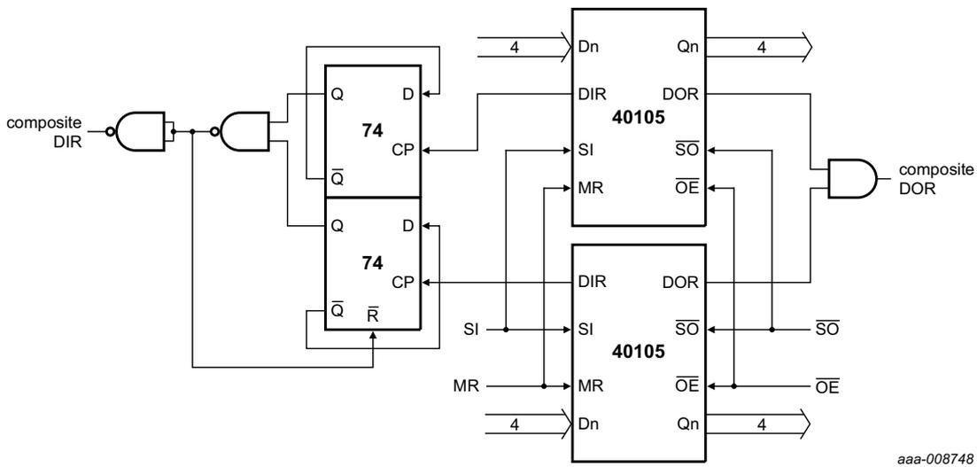
This circuit is only required if the SI input is constantly held HIGH, when the FIFO is empty and the automatic shift-in cycles are started (see Figure 9).
