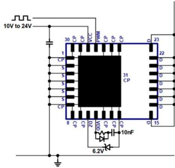
Fig. 18. Start-up circuit
