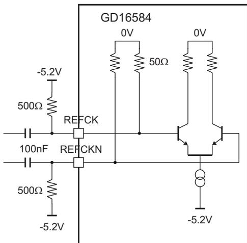
Figure 6. Reference Clock Input (REFCK/REFCKN), Differential AC Coupled.
