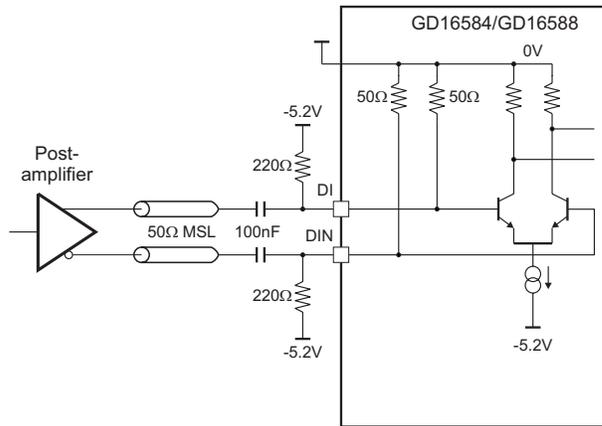
Figure 4. 10 Gbit/s Input (DI/DIN), AC Coupled
