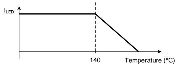
**Figure 5: I<sub>LED</sub> Decreases with Temperature**
