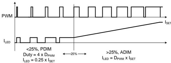
**Figure 2: Mix Dimming with 25% Transfer Point**
