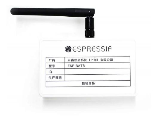
During the production testing, the signal board can be used as a standard device for communication with the DUT (Provided by Espressif).
