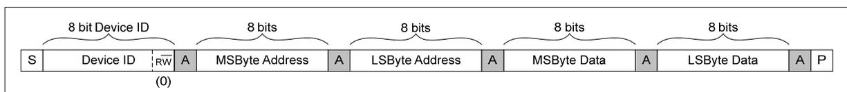
Figure 9 Single Register Write to Specified Address
