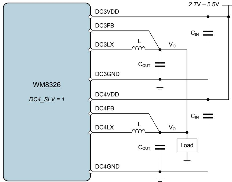
Figure 21 DC-DC3 / DC-DC4 Dual Mode Converter Connections
