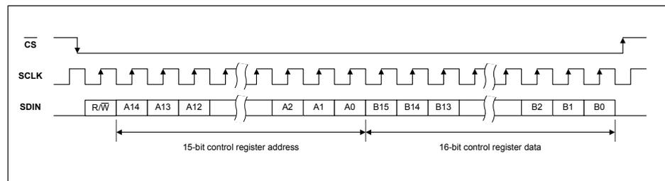
Figure 14 Control Interface 4-wire (SPI) Register Write
