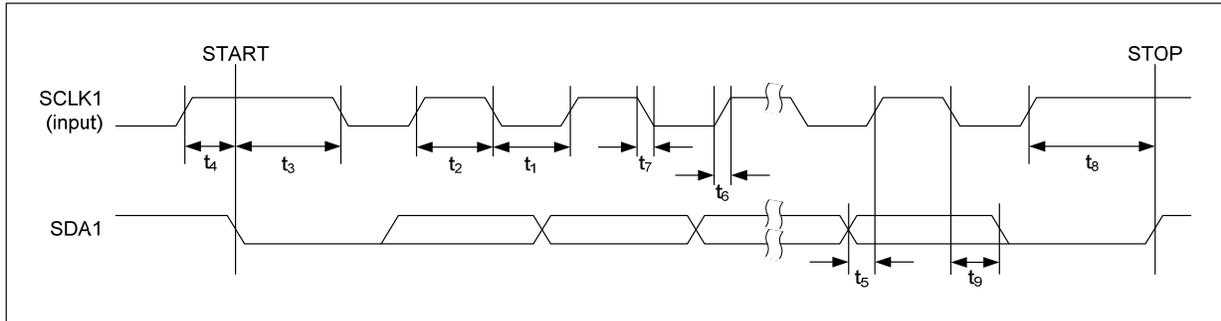
Figure 1 Control Interface Timing - 2-wire (I2C) Control Mode
