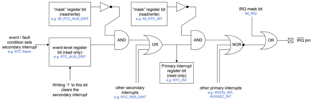
Figure 24 Interrupt Logic
