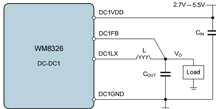
Note: Equivalent circuit applies for DC-DC2, DC-DC3 and DC-DC4
