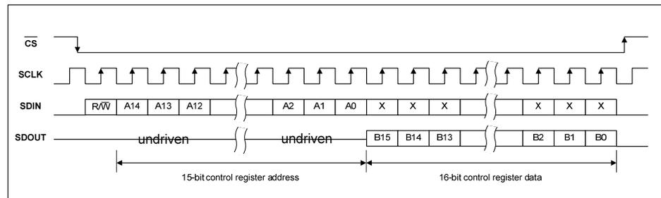
Figure 15 Control Interface 4-wire (SPI) Register Read
