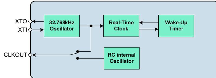
**Figure 16** Clocking Configuration
