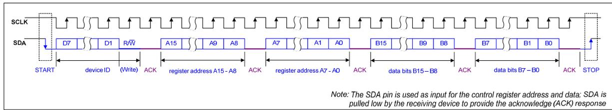
Figure 7 Control Interface 2-wire (I2C) Register Write
