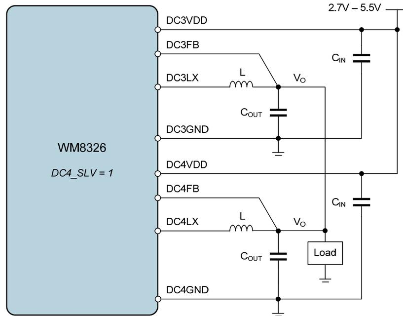
Figure 30 DC-DC3 / DC-DC4 Dual Mode Converter Connections
