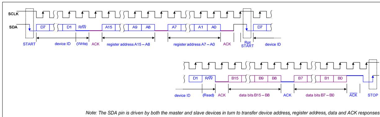
Figure 8 Control Interface 2-wire (I2C) Register Read
