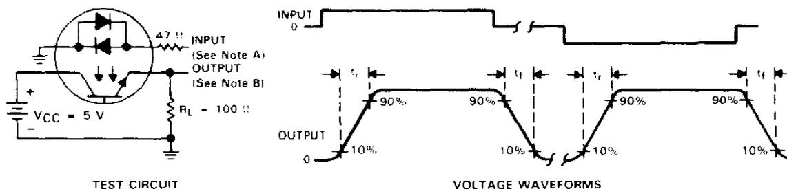
NOTES A The input waveform is supplied by a generator with the following characteristics:  $Z_0 = 50\ \Omega$ ,  $t_r \leq 15\text{ ns}$ , duty cycle = 1%
