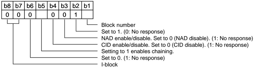
Figure 4-16 I-block Coding
