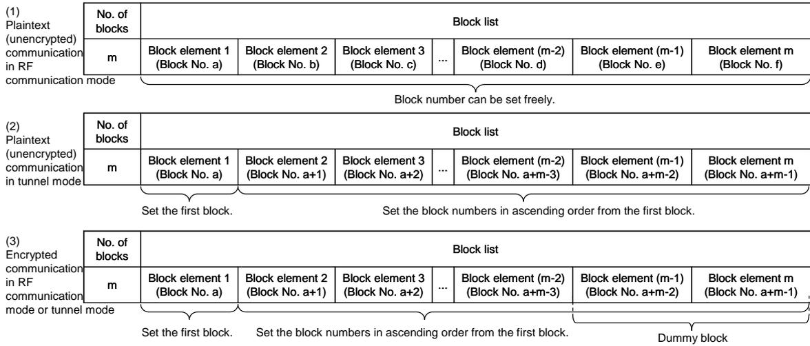
Figure 4-11 Block List Referenced from this RFID
