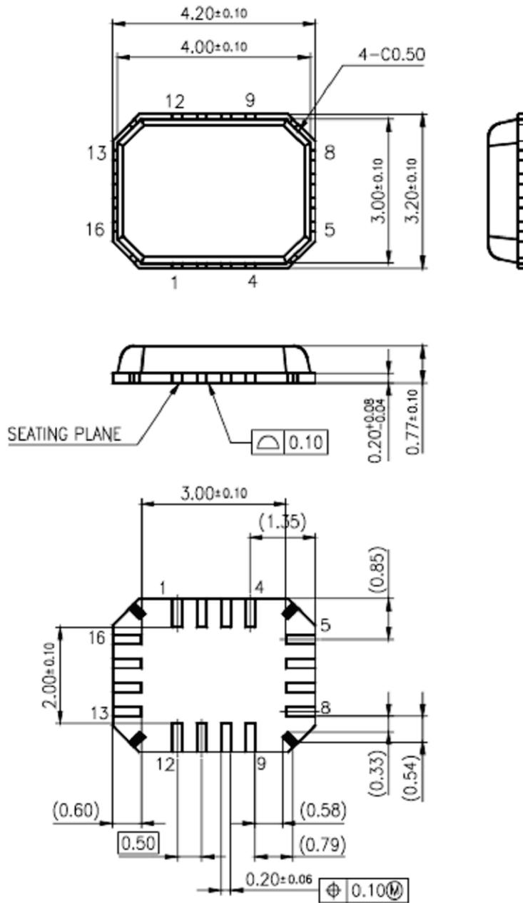
Figure 2-2 Outside drawing (QFN016)
