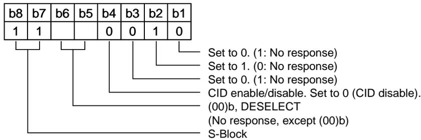
Figure 4-18 S-block Coding
