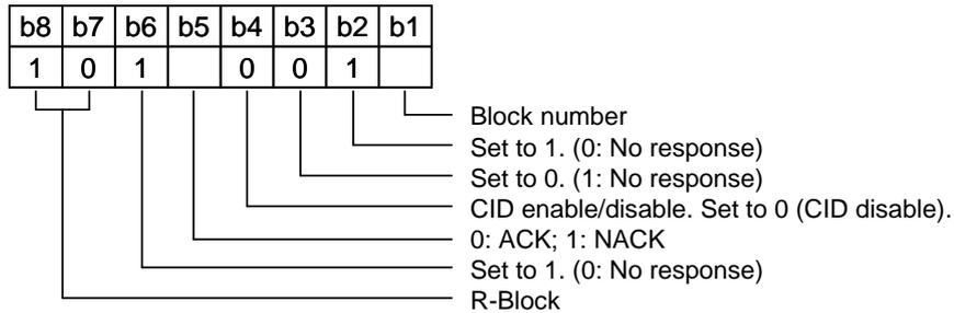
Figure 4-17 R-block Coding
