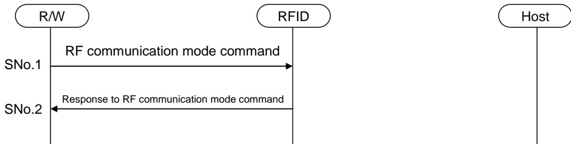
Figure 4-1 RF Communication Mode Sequence
