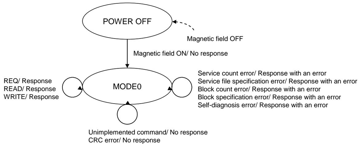
Figure 4-3 State Transition Diagram of JISX6319-4 PICC
