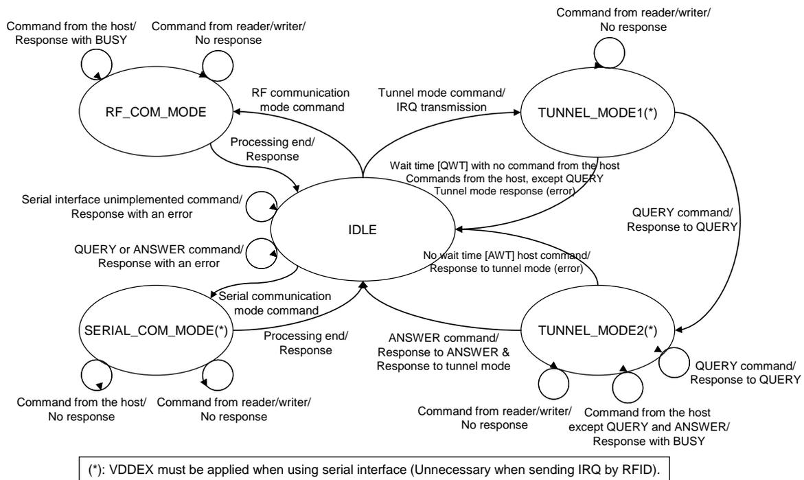
Figure 8-3 State Transition Diagram in Operation Mode
