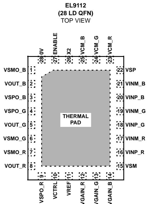
EXPOSED DIEPLATE SHOULD BE CONNECTED TO -5V
