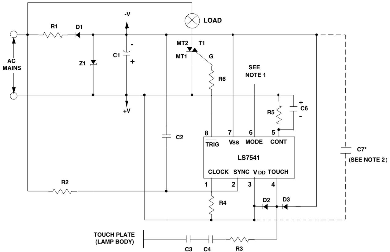
The Figure 5 Application Schematic functions identically to that shown in Figure 4 with one less component. Referencing Triac T1 to the +V power supply of the IC eliminates the need to AC couple the TRIAC pulse to the Triac Gate thereby eliminating component C5.
