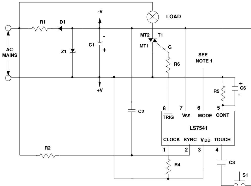
Using the Figure 5 schematic as an example, components R3, C4, C7, D1 and D2 are eliminated and Pushbutton Switch, S1, is connected from one end of C3 to Vss. Each depression of S1 causes the Brightness Level to change in the same way as a Touch does in Figure 5. C3 is 1000pf, 10V capacitor.
