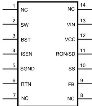
**Figure 1. 14-Lead HTSSOP (Top View)**
