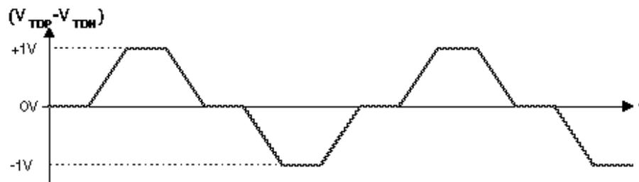
The magnetics module external to the 82562EZ converts  $I_{TDP}$  and  $I_{TDN}$  to  $2.0 V_{PP}$  as required by the TP-PMD specification. The same magnetics used for 100BASE-TX mode can also work in 10BASE-T mode.
