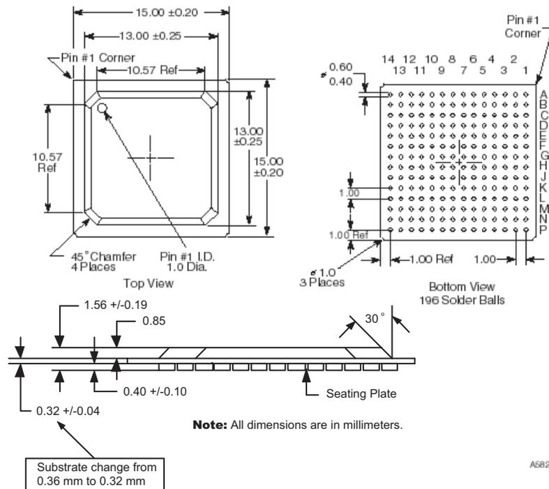
**Note:** No changes to existing soldering processes are needed for the 0.32 mm substrate change.
