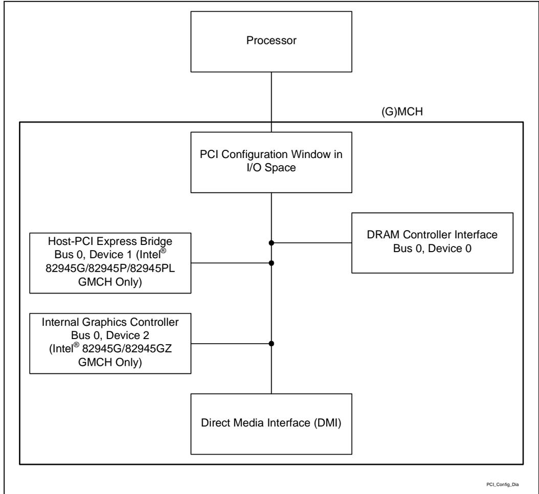
The (G)MCH contains three PCI devices within a single physical component. The configuration registers for the three devices are mapped as devices residing on PCI bus 0.
