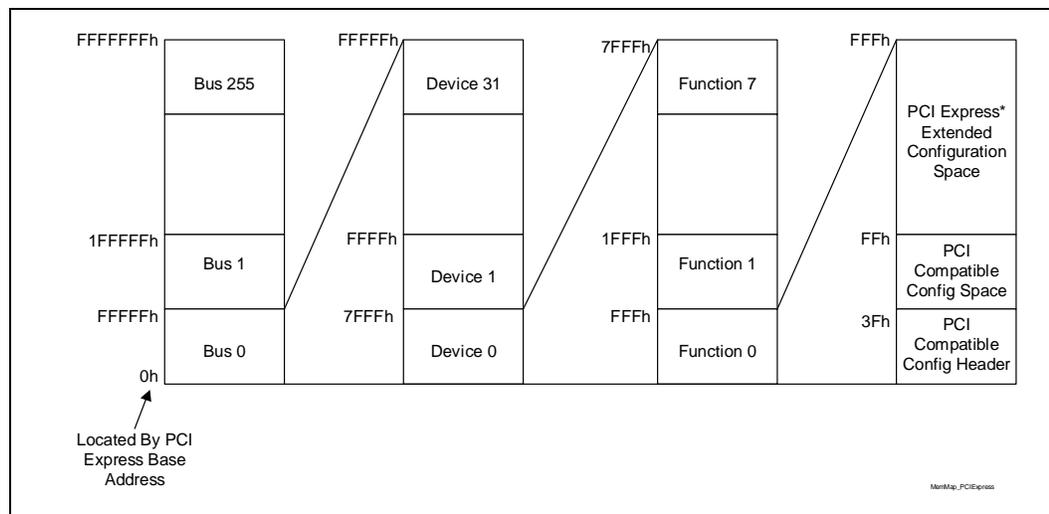
As with PCI devices, each PCI Express device is selected based on decoded address information that is provided as a part of the address portion of configuration request packets. A PCI Express device will decode all address information fields (bus, device, function, and extended address numbers) to provide access to the correct register.
