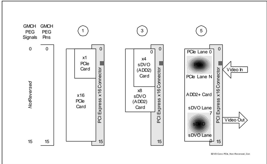
Figure 10-4. Concurrent SDVO / PCI Express\* Reversed Configurations
