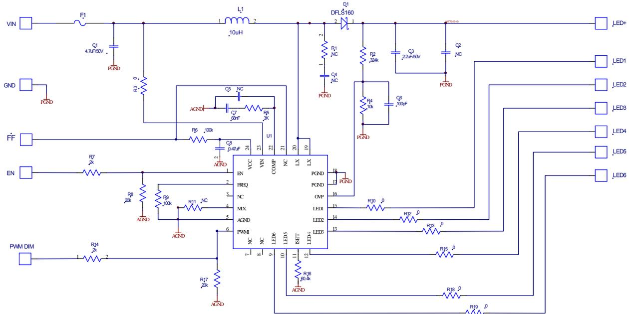
**Figure 1:  $V_{IN} > 5.5V$ , 6string, 20mA/string application**
