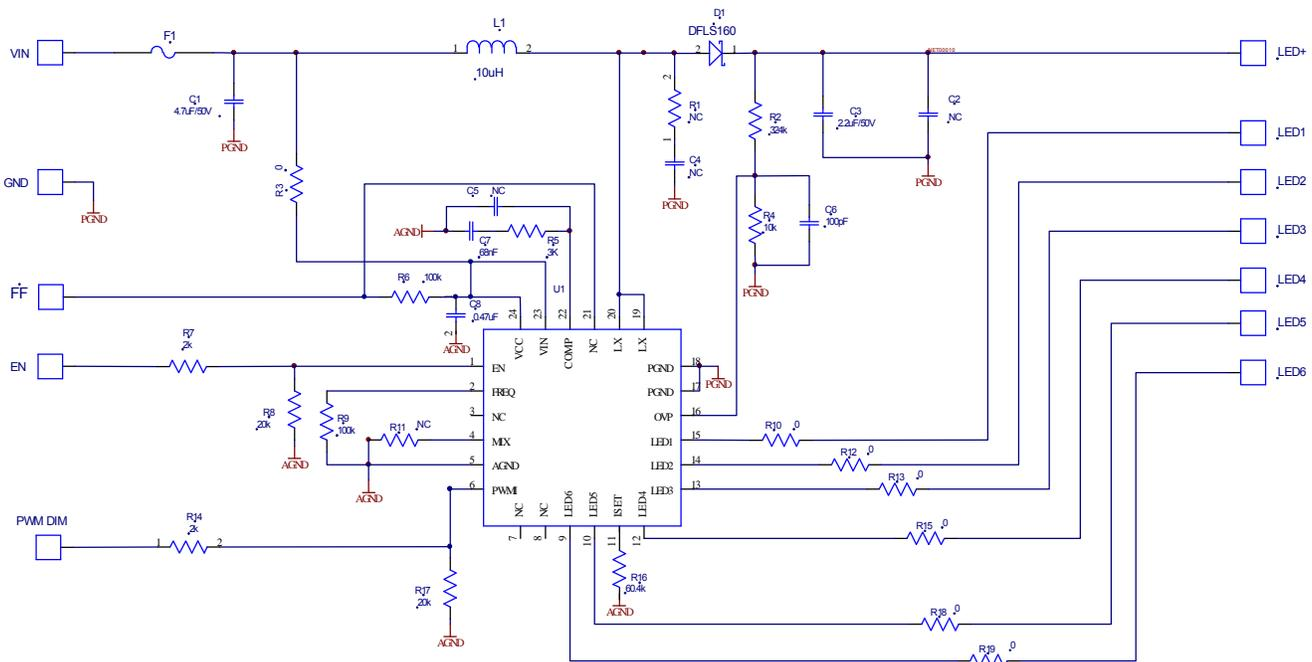
**Figure 2:  $V_{IN} < 5.5V$ , 6string, 20mA/string application**
