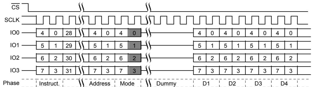
**Figure 4.11 DDR Quad I/O Read**
