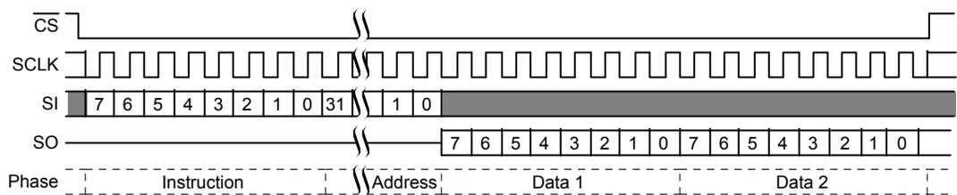
**Figure 4.7** Single Bit Wide I/O Command with latency
