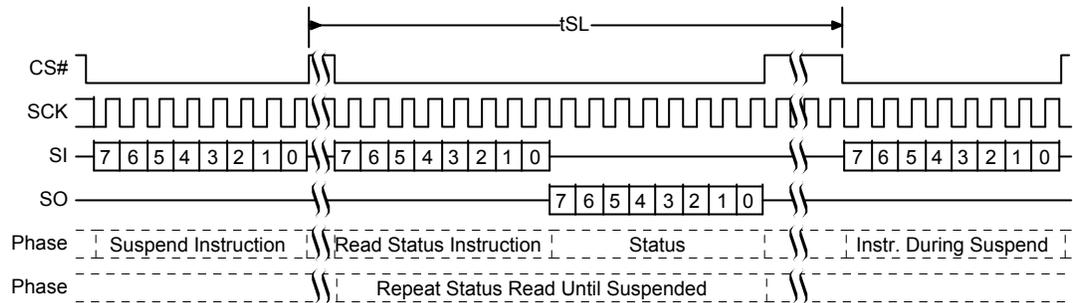
**Figure 10.46** Erase or Program Suspend Command Sequence
