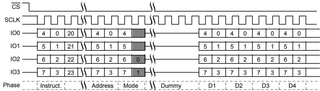
**Figure 10.26** Continuous Quad I/O Read Command Sequence (3-Byte Address)
