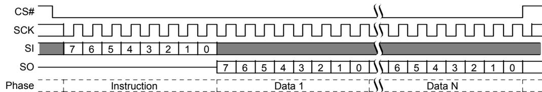
This command is also supported in QPI mode. In Quad All mode the instruction is shifted in on IO0-IO3 and the returning data is shifted out on IO0-IO3.
