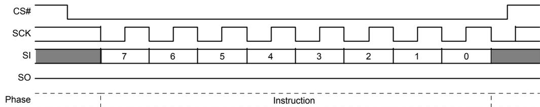
**Figure 10.49** Erase or Program Resume Command Sequence QPI Mode
