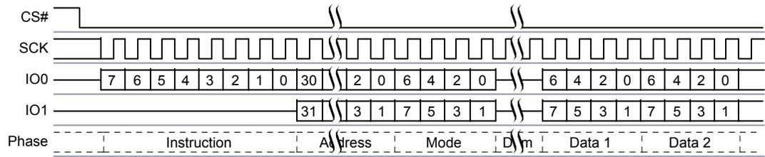
**Figure 4.9 Quad I/O Command**
