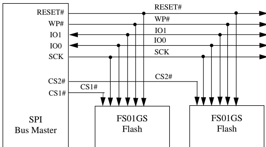
**Figure 3.3** Bus Master and Memory Devices on the SPI Bus - Quad Bit Data Path
