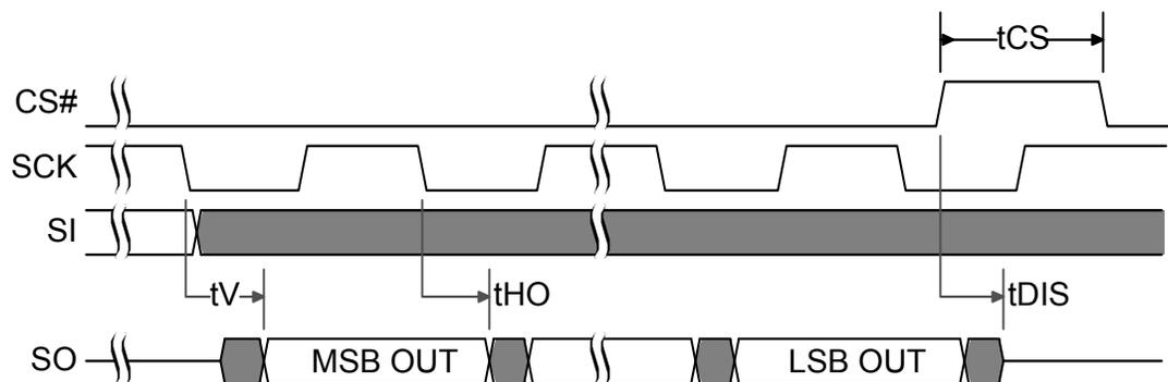
**Figure 6.12** SPI SDR MIO Timing
