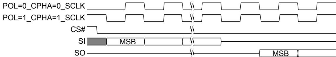
Timing diagrams throughout the remainder of the document are generally shown as both mode 0 and 3 by showing SCK as both high and low at the fall of CS#. In some cases a timing diagram may show only mode 0 with SCK low at the fall of CS#. In such a case, mode 3 timing simply means clock is high at the fall of CS# so no SCK rising edge set up or hold time to the falling edge of CS# is needed for mode 3.
