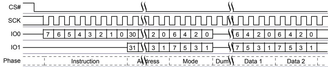
**Figure 10.23** Dual I/O Continuous Read Command Sequence (4-Byte Address [CR2V[7]=1])
