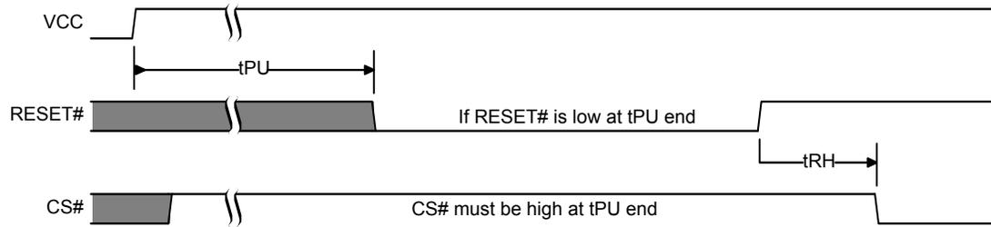
**Figure 6.5** Reset high at the end of POR
