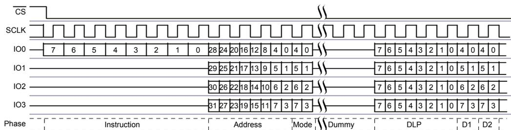
**Figure 4.12** DDR Quad I/O Read in QPI Mode
