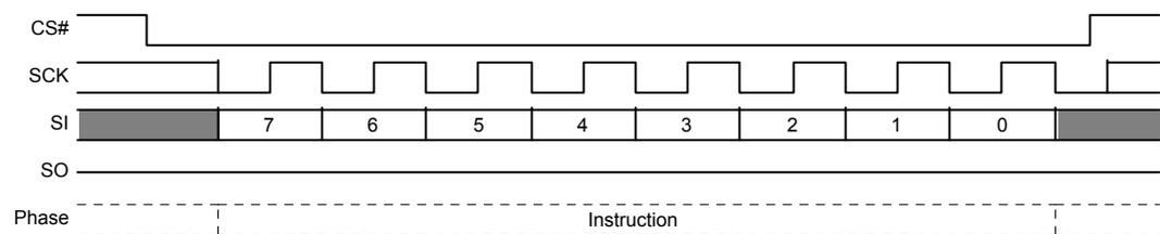
This command is also supported in QPI mode. In Quad All mode the instruction is shifted in on IO0-IO3, two clock cycles per byte.
