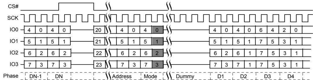
**Figure 10.27** Quad I/O Read Command Sequence (4-Byte Address, ECh or EBh [CR2V[7]=1])
