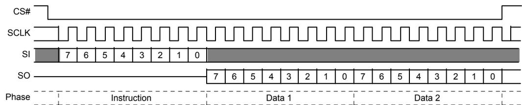
**Figure 4.6** Single Bit Wide I/O Command without latency
