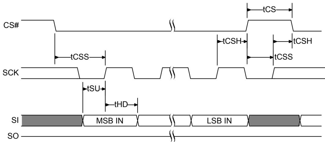
Figure 6.11 SPI Single Bit Output Timing
