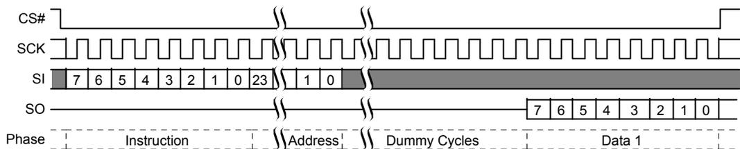
This command is also supported in QPI mode. In Quad All mode the instruction is shifted in on IO0-IO3 and the returning data is shifted out on IO0-IO3.
