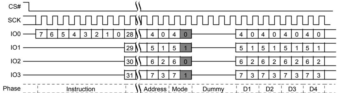
**Figure 10.28** Continuous Quad I/O Read Command Sequence (4-Byte Address)
