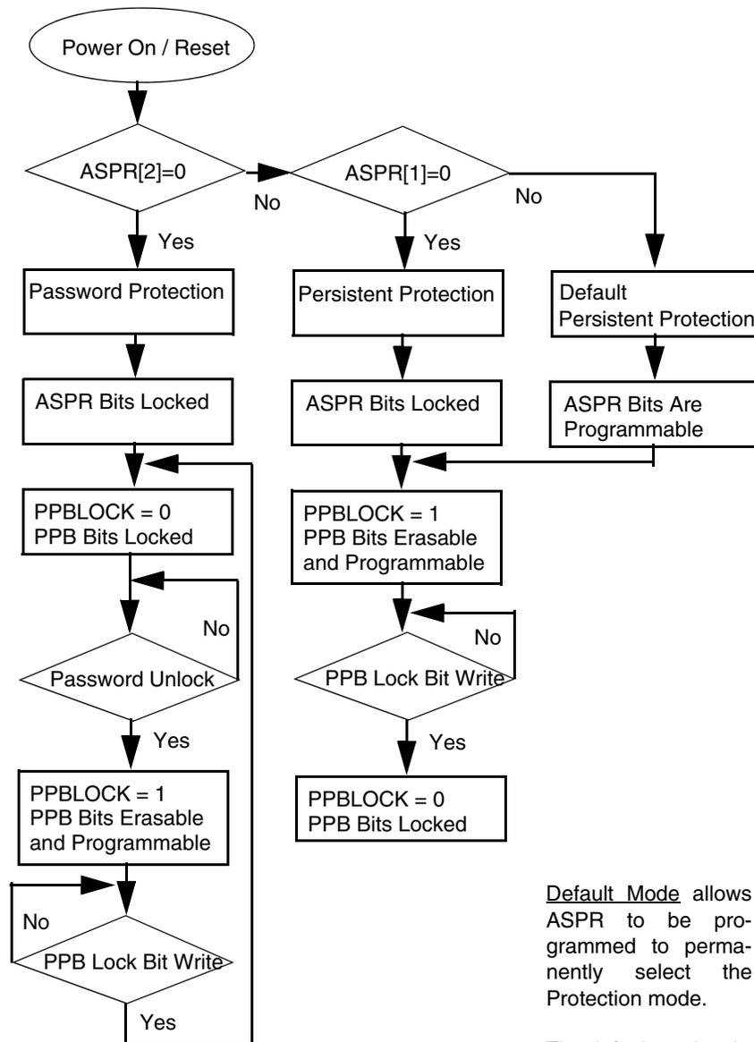
Password Protection Mode protects the PPB after power up. A password unlock command will enable changes to PPB. A PPB Lock Bit write command turns protection back on.
