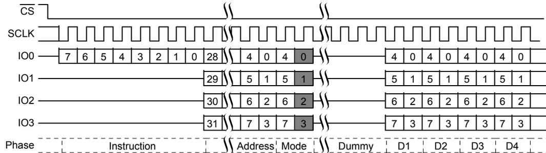
**Figure 4.10 Quad I/O Read Command in QPI Mode**
