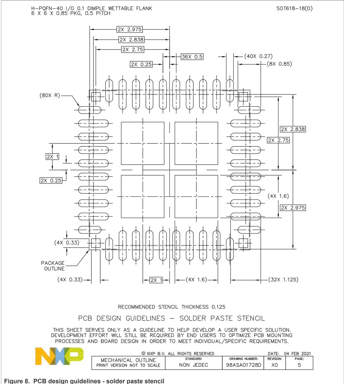
Figure 8. PCB design guidelines - solder paste stencil
