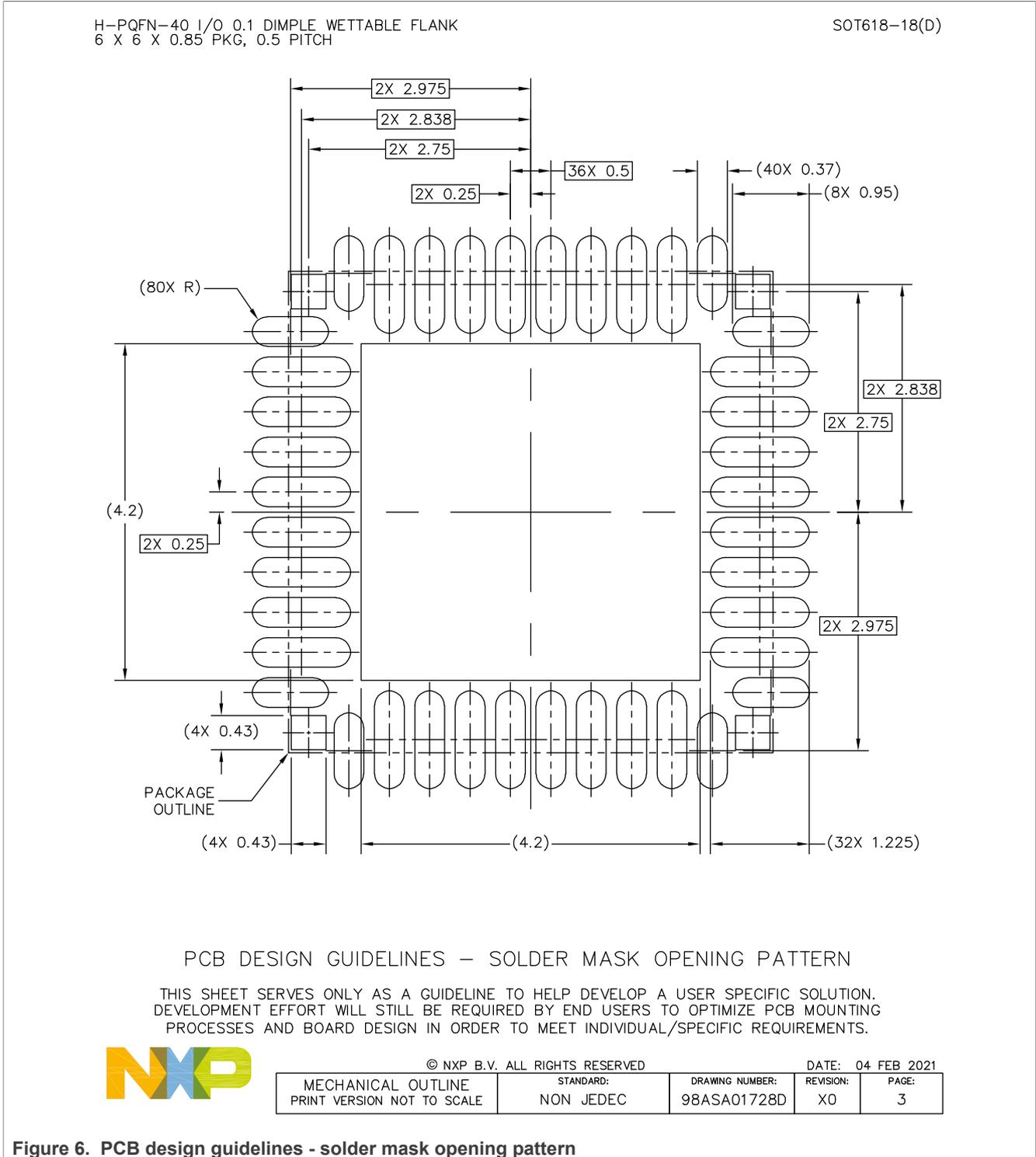
Figure 6. PCB design guidelines - solder mask opening pattern
