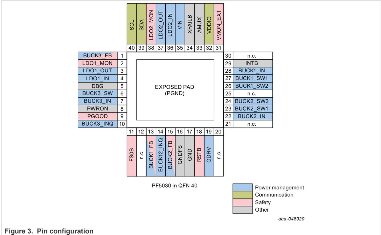
Figure 3. Pin configuration
