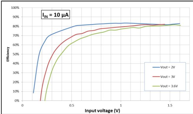
Figure 7-1 Charger Efficiency vs Input Voltage ( $I_{IN} = 10\mu A$ )
