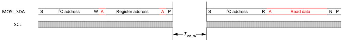
**Figure 6-11 I<sup>2</sup>C transaction for reading the E<sup>2</sup>PROM**
