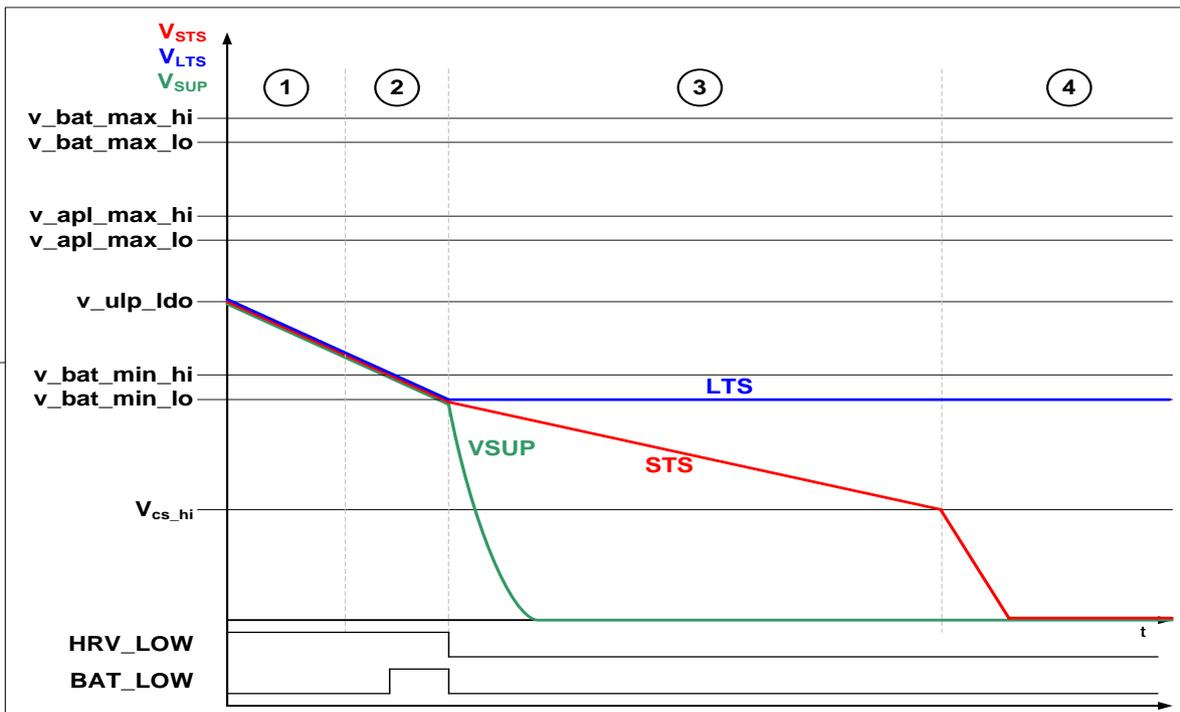
Figure 1-5 Application shut-down without energy from the harvester
