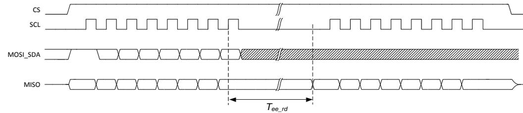
**Figure 6-7 SPI transaction for reading the E<sup>2</sup>PROM (CPOL=0)**
