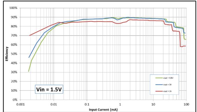
Figure 7-2 Charger Efficiency vs Input Current ( $V_{IN} = 1.5V$ )
