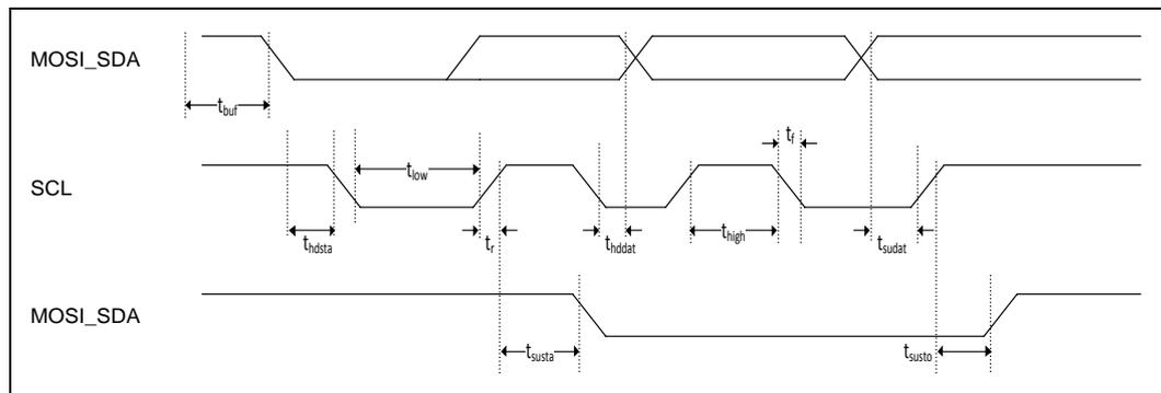
Figure 4-2 I<sup>2</sup>C Timing Diagram
