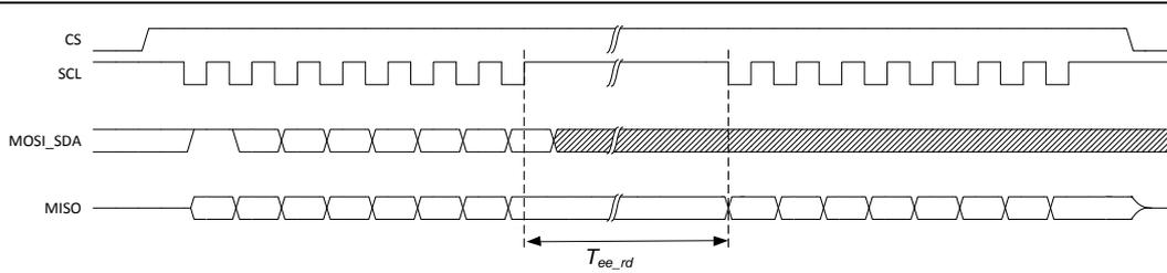
**Figure 6-6 SPI transaction for reading the E<sup>2</sup>PROM (CPOL=1)**
