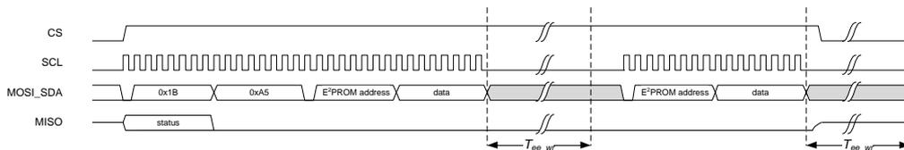
**Figure 6-9 SPI multi-byte transaction for writing the E<sup>2</sup>PROM**
