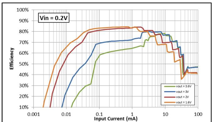
Figure 7-6 Charger Efficiency vs Input Current ( $V_{IN} = 0.2V$ )
