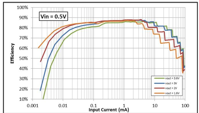
Figure 7-4 Charger Efficiency vs Input Current ( $V_{IN} = 0.5V$ )
