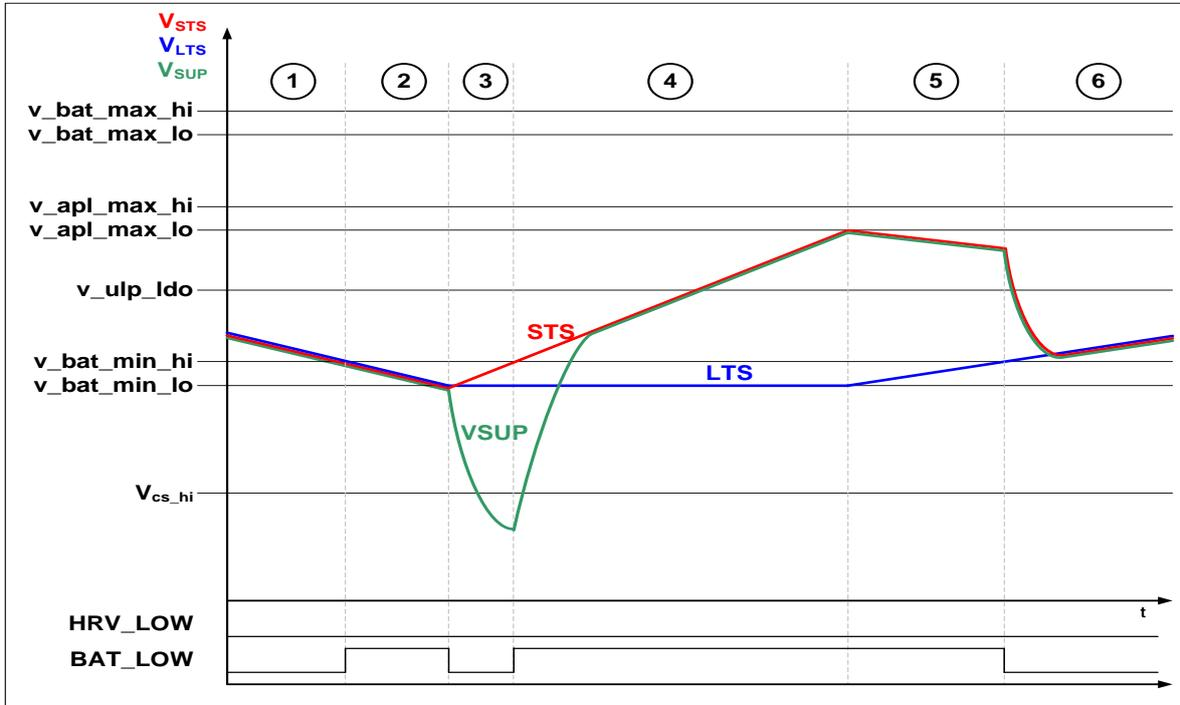
Figure 1-4 Application shut-down with a working harvester
