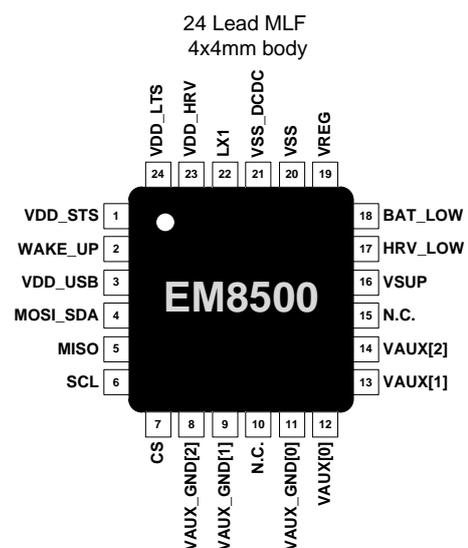
Figure 1-1 QFN24 Package
