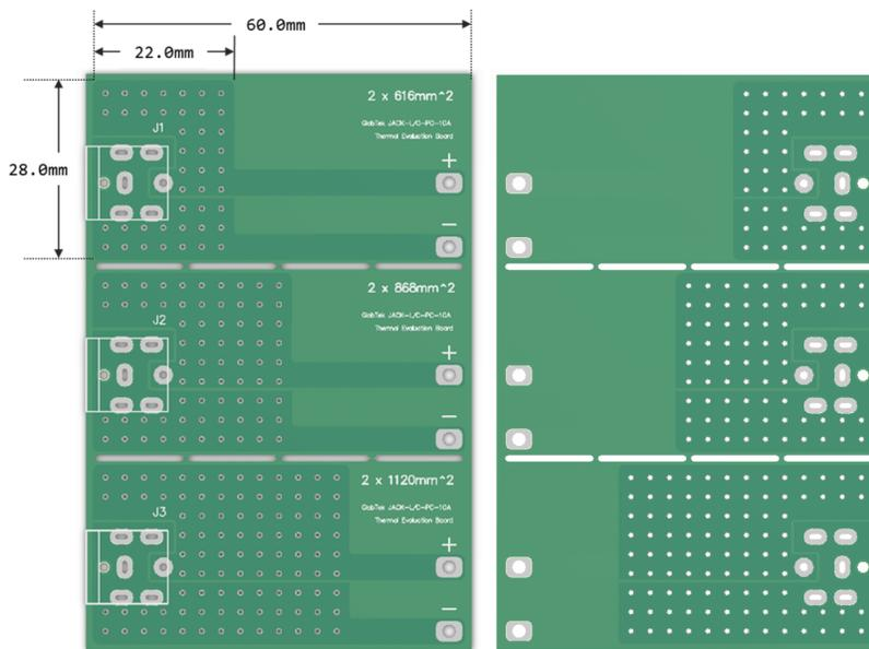
Above: GlobTek Thermal Evaluation Board for JACK-L-PC-10A-RA(R) and JACK-C-PC-10A-RA(R)
