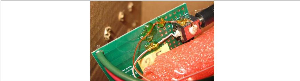
Note, maximum hotspot temperature on the PCB will be approximately 10°C cooler than the hot spot on the center pin, due to thermal gradient along the pin length as it merges into the large copper plane area.
