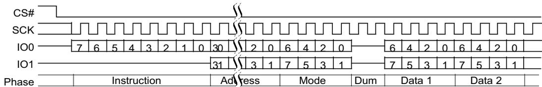
**Figure 10.34** Continuous Dual I/O Read Command Sequence (4-Byte Address, BCh or BBh [ExtAdd=1], EHPLC=10b)
