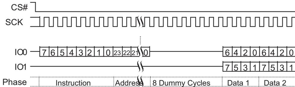
**Figure 10.27** Dual Output Read Command Sequence
