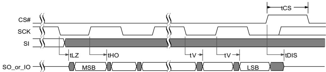
Figure 6.16 SPI DDR Data Valid Window
