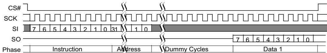
Figure 4.8 Dual Output Command
