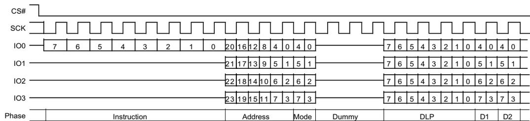
**Figure 10.48** Continuous DDR Quad I/O Read Subsequent Access (3-Byte Address, HPLC=11b)
