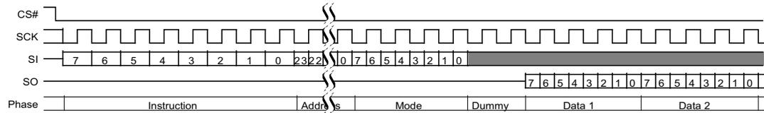
**Figure 10.40** Continuous DDR Fast Read Subsequent Access (3-Byte Address [ExtAdd=0, EHPLC=11b])
