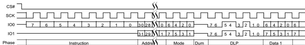
**Figure 10.45** Continuous DDR Dual I/O Read Subsequent Access (4-Byte Address, EHPLC= 01b)
