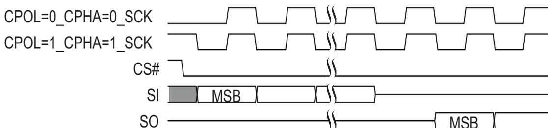
Timing diagrams throughout the remainder of the document are generally shown as both mode 0 and 3 by showing SCK as both high and low at the fall of CS#. In some cases a timing diagram may show only mode 0 with SCK low at the fall of CS#. In such a case, mode 3 timing simply means clock is high at the fall of CS# so no SCK rising edge set up or hold time to the falling edge of CS# is needed for mode 3.
