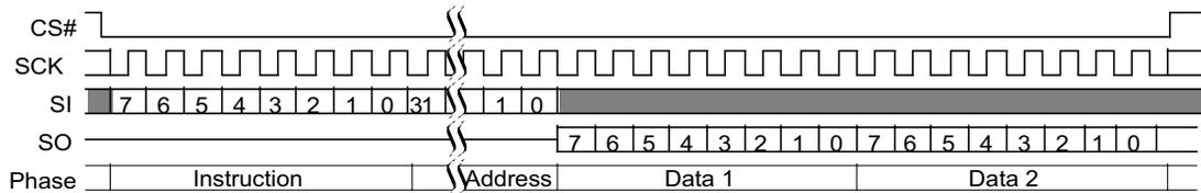
**Figure 4.7** Single Bit Wide I/O Command with Latency
