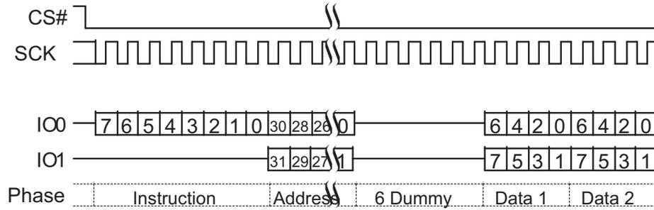
Figure 4.9 Quad Output Command without Latency
