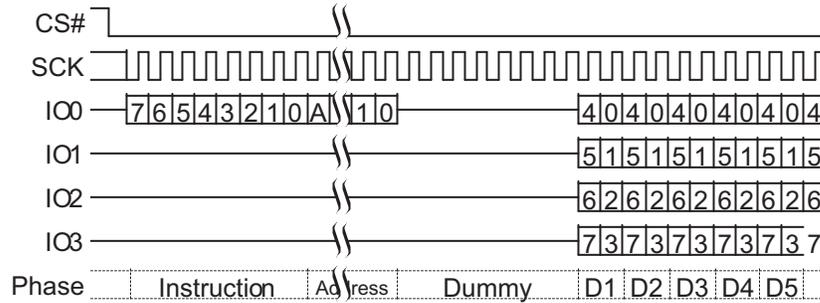
Figure 10.30 Quad Output Read (QOR 6Bh or 4QOR 6Ch) Command Sequence without Read Latency
