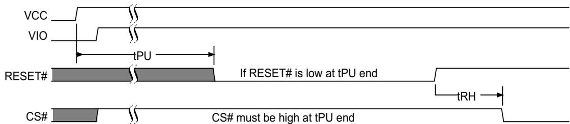
Figure 6.5 Reset High at the End of POR
