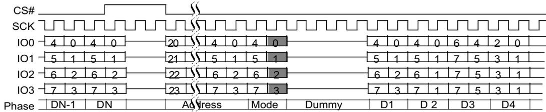
**Figure 10.37** Quad I/O Read Command Sequence (4-Byte Address, ECh or EBh [ExtAdd=1], LC=00b)
