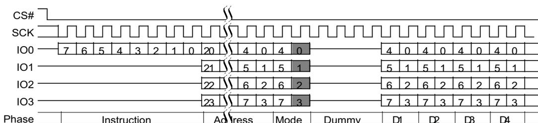
**Figure 10.36** Continuous Quad I/O Read Command Sequence (3-Byte Address), LC=00b
