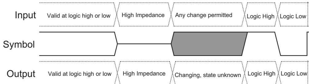
Figure 6.2 Input, Output, and Timing Reference Levels
