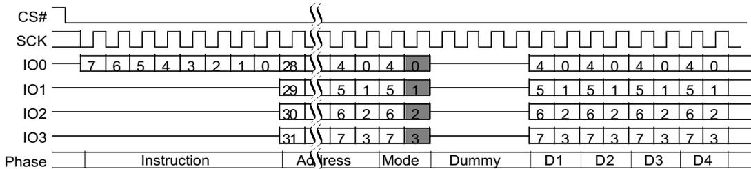
**Figure 10.38** Continuous Quad I/O Read Command Sequence (4-Byte Address), LC=00b
