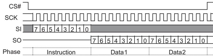
**Figure 4.6** Single Bit Wide I/O Command without Latency
