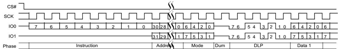
Figure 4.14 DDR Quad I/O Read
