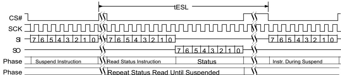
**Figure 10.58 Erase Resume (ERRS 7Ah) Command Sequence**
