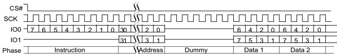
Figure 4.11 Quad I/O Command
