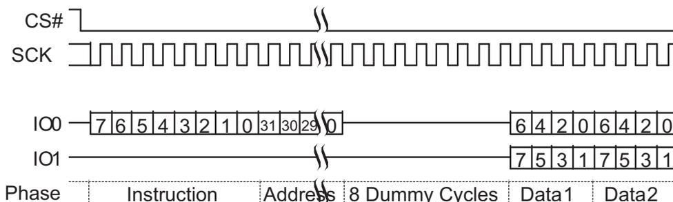
**Figure 10.28** Dual Output Read Command Sequence
