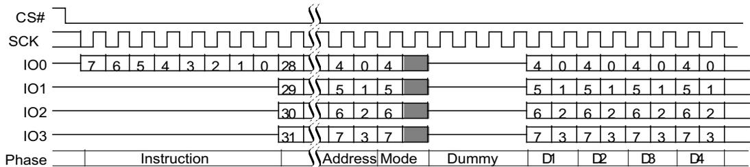
Figure 4.12 DDR Fast Read with EHPLC = 00b
