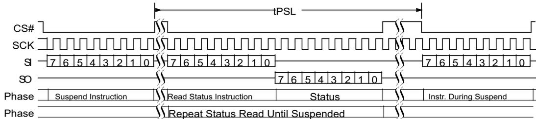
**Figure 10.54** 10.55 Program Resume (PGRS 8Ah) Command Sequence
