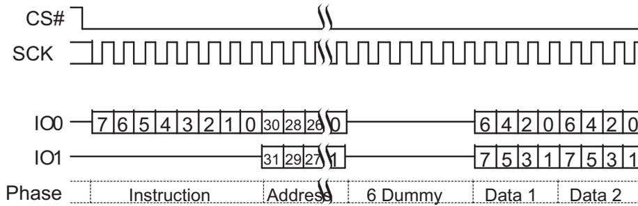
**Figure 10.33** Dual I/O Read Command Sequence (4-Byte Address, BCh or BBh [ExtAdd=1], EHPLC=10b)
