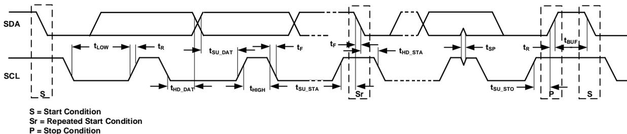
**Figure 4: I<sup>2</sup>C-Compatible Interface Timing Diagram**
