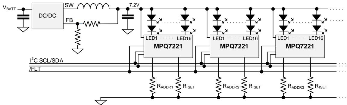
Figure 2: System Application Circuit with 2 LEDs in Series
