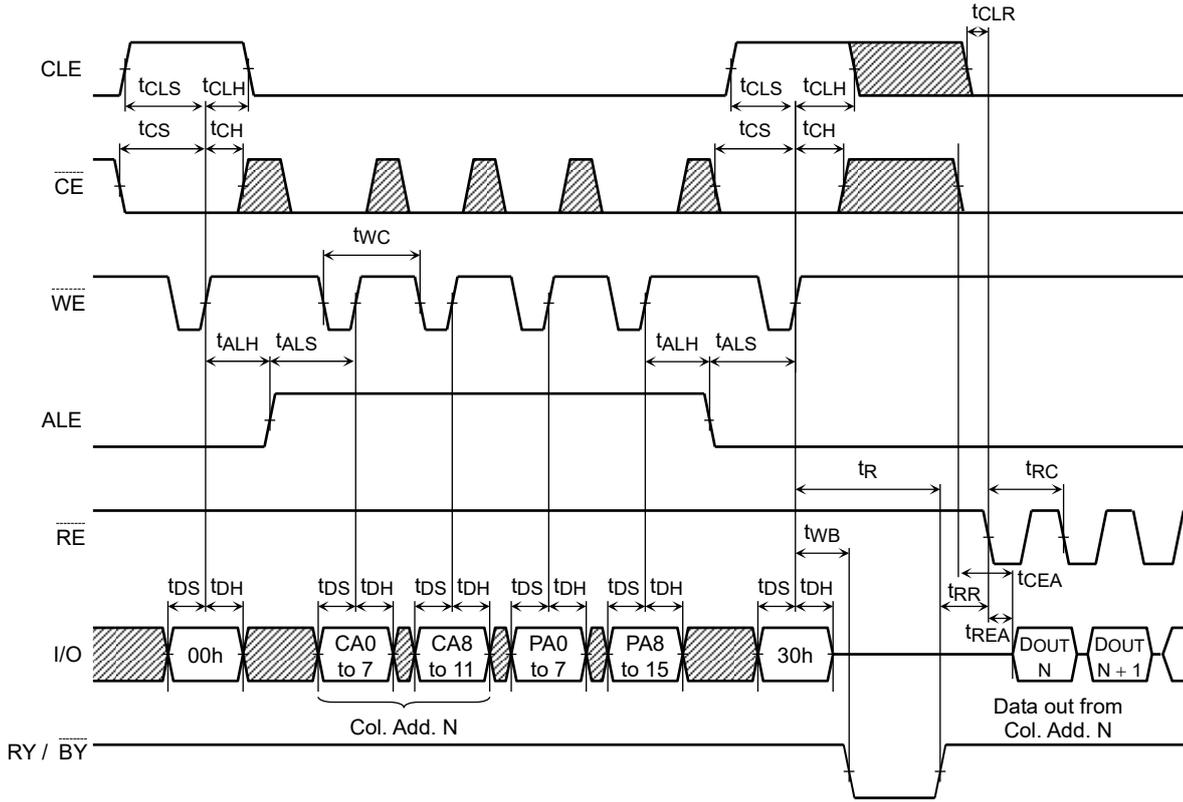
Read Cycle Timing Diagram: When Interrupted by CE
