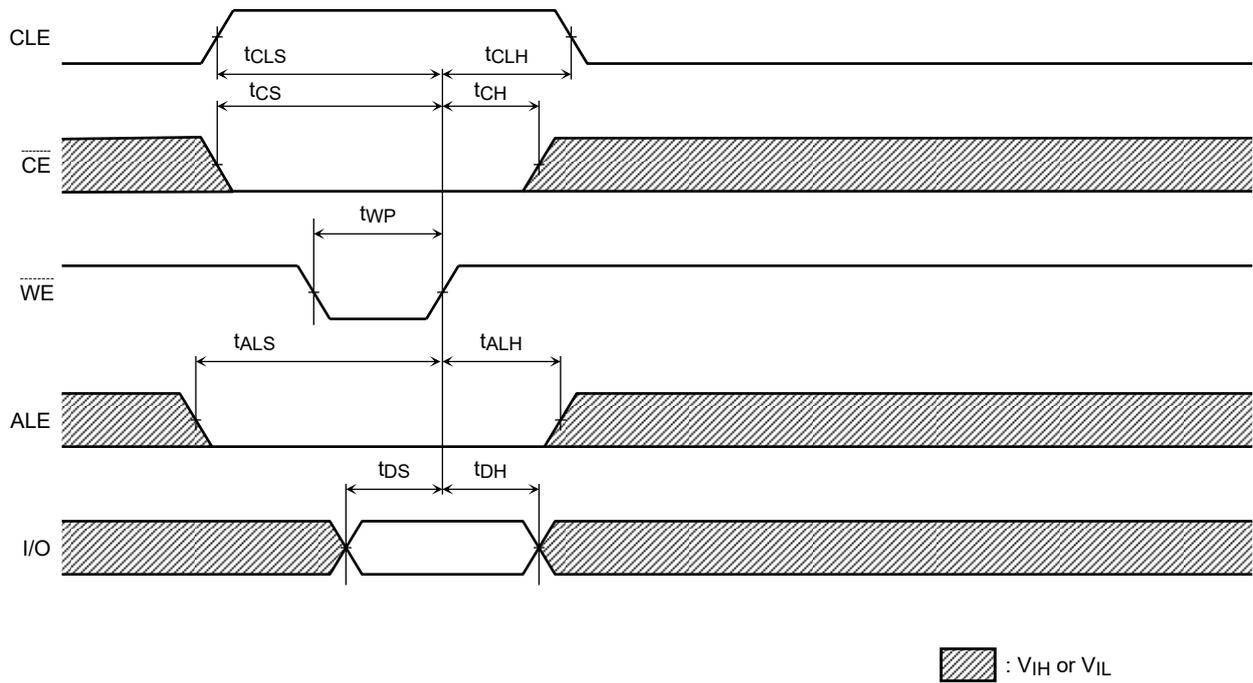
Address Input Cycle Timing Diagram
