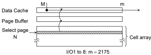
A data transfer operation from the cell array to the Data Cache via Page Buffer starts on the rising edge of WE in the 30h command input cycle (after the address information has been latched). The device will be in the Busy state during this transfer period. After the transfer period, the device returns to Ready state. Serial data can be output synchronously with the RE clock from the start address designated in the address input cycle.
