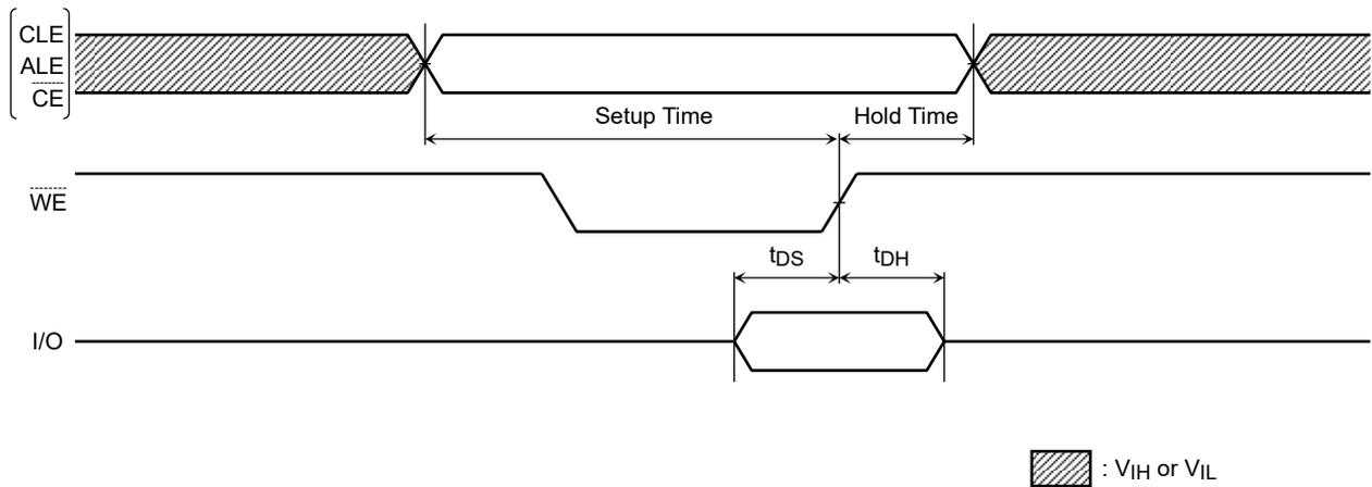
Command Input Cycle Timing Diagram
