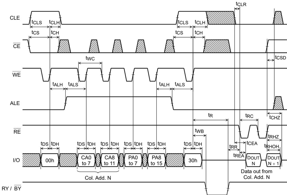
Read Cycle with Data Cache Timing Diagram (1/2)
