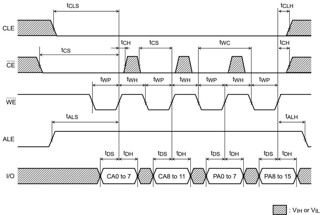
Data Input Cycle Timing Diagram
