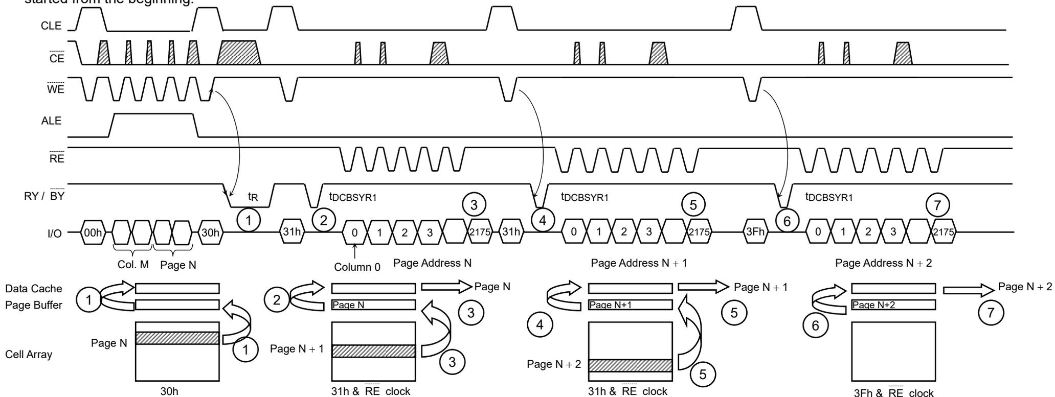
If the 31h command is issued to the device, the data content of the next page is transferred to the Page Buffer during serial data out from the Data Cache, reducing the  $t_{\text{R}}$  (Data transfer from memory cell to data register).
