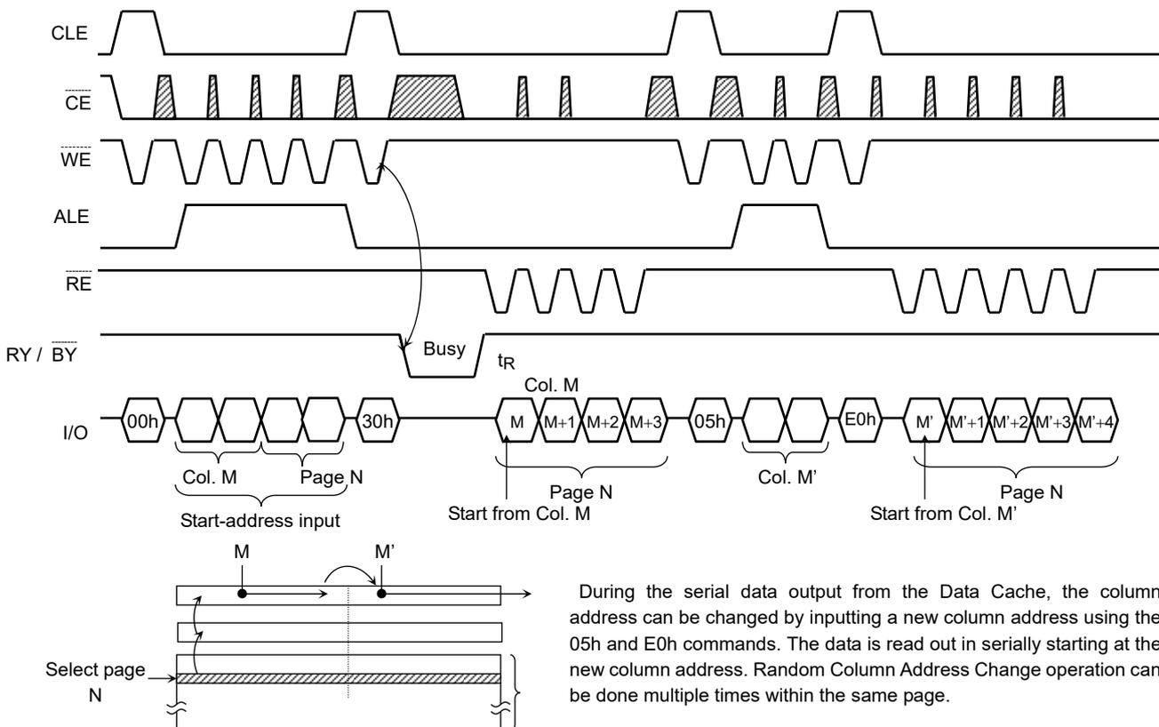
During the serial data output from the Data Cache, the column address can be changed by inputting a new column address using the 05h and E0h commands. The data is read out in serially starting at the new column address. Random Column Address Change operation can be done multiple times within the same page.
