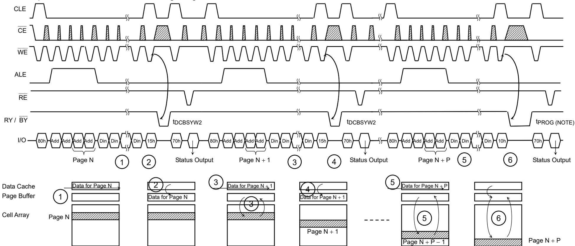
Issuing the 15h command to the device after serial data input initiates the program operation with Data Cache
