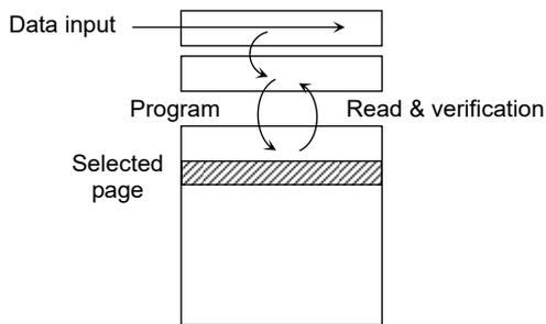
The data is transferred (programmed) from the Data Cache via the Page Buffer to the selected page on the rising edge of WE following input of the "10h" command. After programming, the programmed data is transferred back to the register to be automatically verified by the device. If the programming does not succeed, the Program/Verify operation is repeated by the device until success is achieved or until the maximum loop number set in the device is reached.
