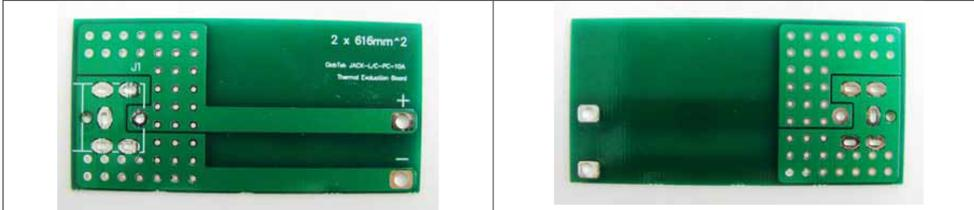
GLOBTEK RECOMMENDED MOUNTING BOARD FOR THE CONNECTORS
