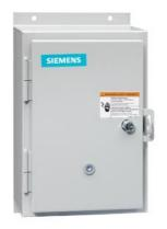
Non-reversing motor starter, Size 0, Three phase full voltage, Solid-state overload relay, OLRelay amp range 0.25-1a, 380 440/440 480V 50/60HZ coil, Non-combination type, Enclosure type 12, Dust/drip proof for indoors, Extra-wide enclosure
