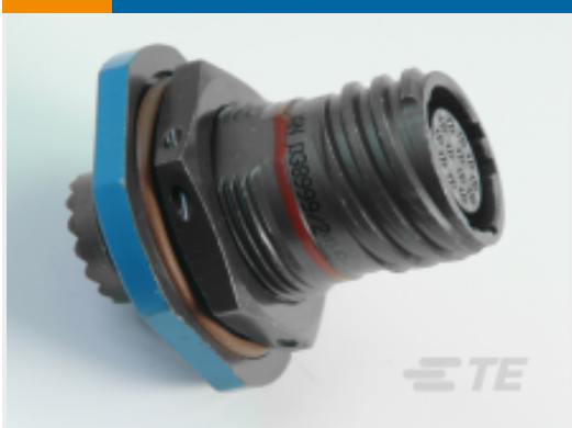
TE Part #YDTS24F23-55SCV001 D38999: Jam Nut, 23-55 Insert, Electroless Nickel Plating
