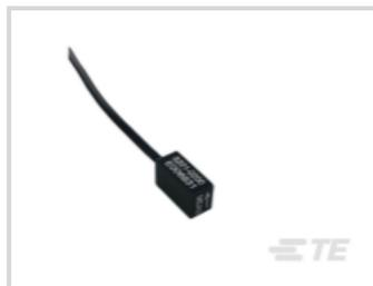
Accelerometer Type: **3-Wire Voltage**Vibration Sensor Product Type: **Piezoelectric Accelerometer**Number of Sensing Axes: **Uniaxial**Frequency Response: **2-10000 Hz**Full Scale Output Voltage: **±1.25 VDC**
