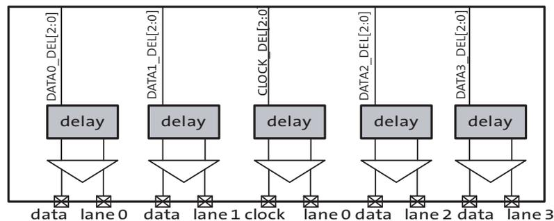
**Figure 11: Delaying the Clock with Respect to Data**
