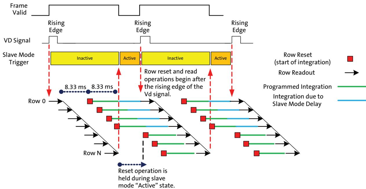
When the slave mode becomes active, the sensor will pause both row read and row reset operations. (Note: The row integration period is defined as the period from row reset to row read.) The frame-time should therefore be configured so that the slave mode “wait period” is as short as possible. In the case where the sensor integration time is shorter than the frame time, the “wait period” will only increase the integration of the rows that have been reset following the last VD pulse.
