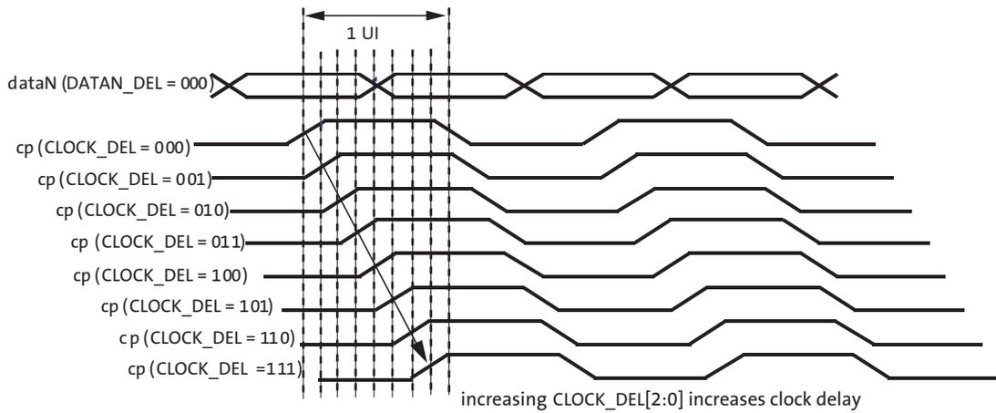
**Figure 12: Delaying Data with Respect to the Clock**
