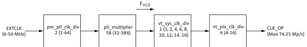
The maximum output of the parallel interface is 74.25 MPixel/s. The sensor will not use the  $F_{SERIAL}$ ,  $F_{SERIAL\_CLK}$ , or  $CLK\_OP$  when configured to use the parallel interface.
