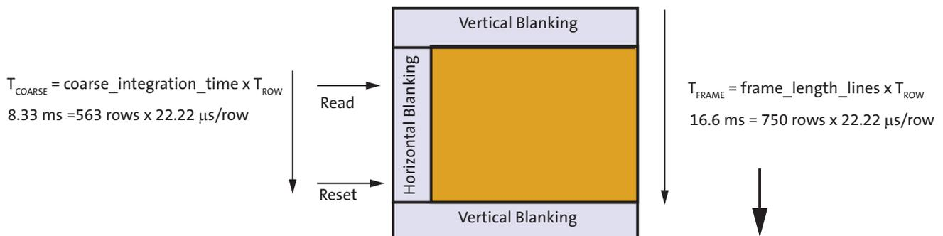
**Figure 15: Row Read and Row Reset Showing Fine Integration**
