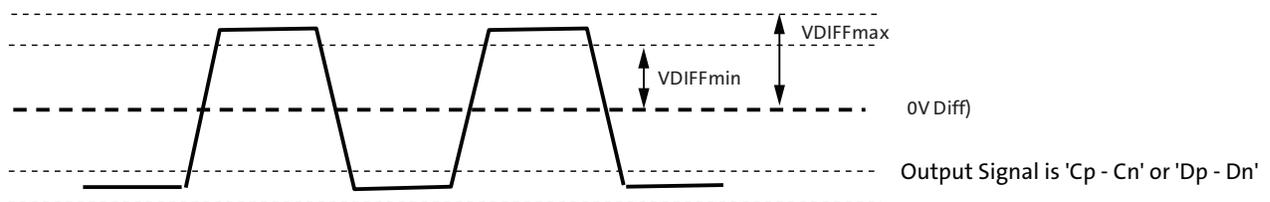
Figure 44: Eye Diagram for Clock and Data Signals
