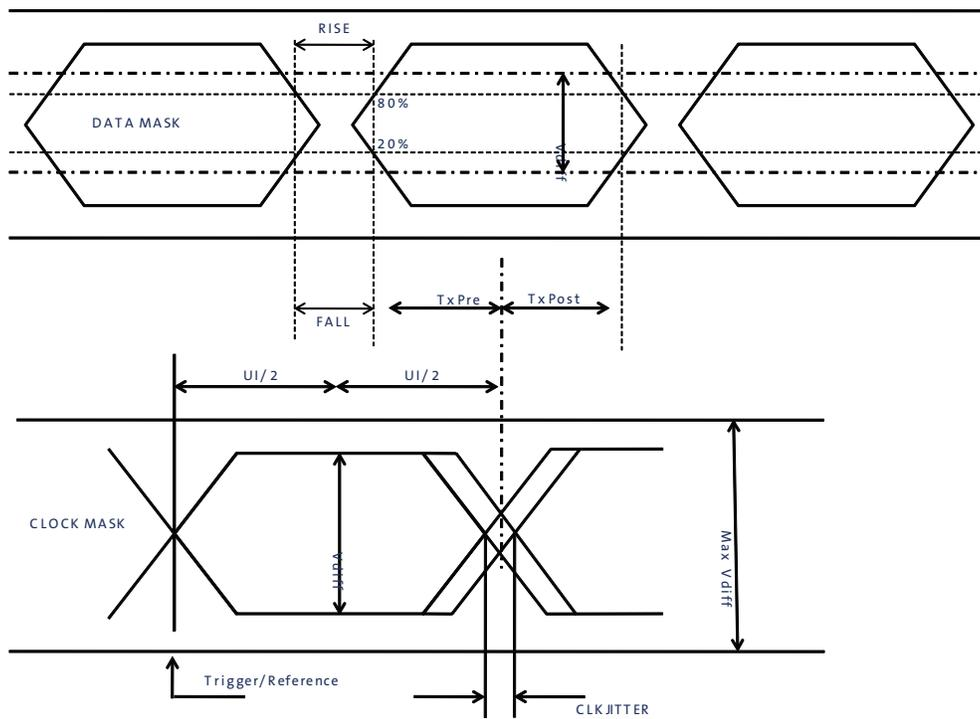
Figure 45: HiSPi Skew Between Data Signals Within the PHY
