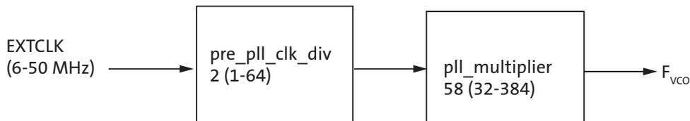
The sensor contains a phase-locked loop (PLL) that is used for timing generation and control. The required VCO clock frequency is attained through the use of a pre-PLL clock divider followed by a multiplier. The PLL multiplier should be an even integer. If an odd integer (M) is programmed, the PLL will default to the lower (M-1) value to maintain an
