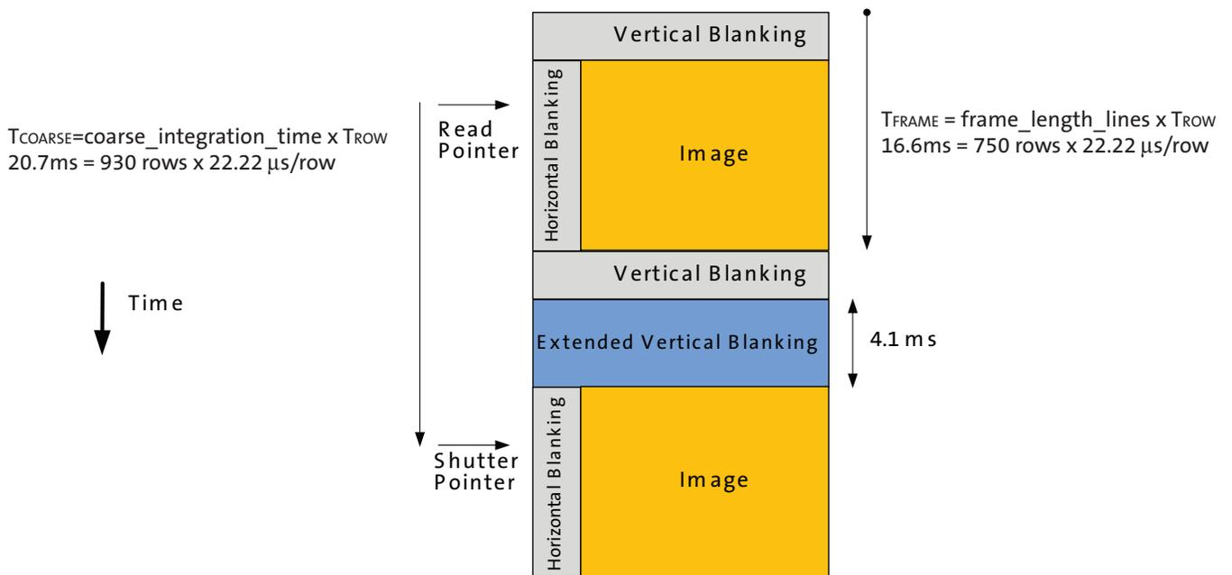
The minimum frame-time is defined by the number of row periods per frame and the row period. The sensor frame-time will increase if the *coarse\_integration\_time* is set to a value equal to or greater than the *frame\_length\_lines*.
