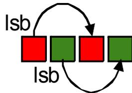
Horizontal binning is achieved either in the pixel readout or the digital readout. The sensor will sample the combined 2x adjacent pixels within the same color plane.
