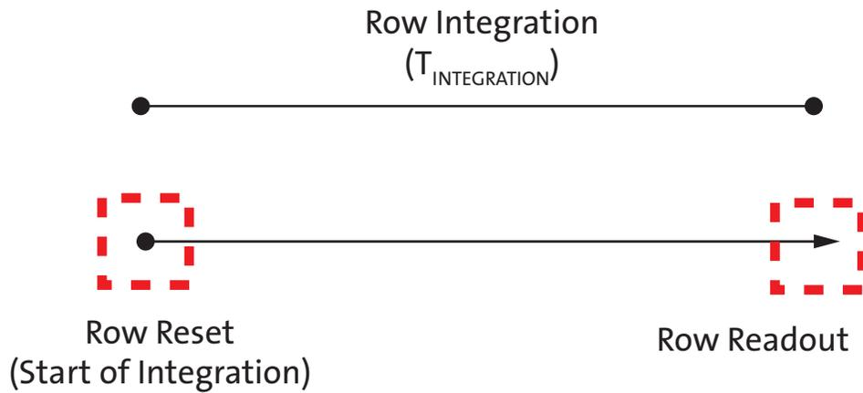
A pixel's integration time is defined by the number of clock periods between a row's reset and read operation. Both the read followed by the reset operations occur within a row period (T<sub>ROW</sub>) where the read and reset may be applied to different rows. The read and reset operations will be applied to the rows of the pixel array in a consecutive order.
