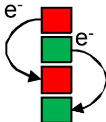
Vertical row binning is applied in the pixel readout. Row binning can be configured as 2x rows within the same color plane.
