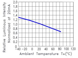
Fig.5 Relative Luminous Intensity vs. Ambient Temperature
