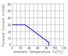
Fig.2 Forward Current Derating Curve
