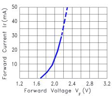
Fig.3 Forward Current vs. Forward Voltage
