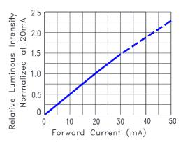
Fig.4 Relative Luminous Intensity vs. Forward Current
