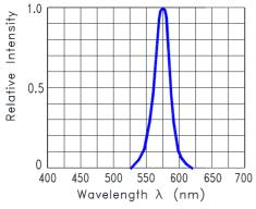
Fig.1 Relative Intensity VS. Wavelength
