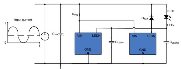
Fig3. Parallel circuit
