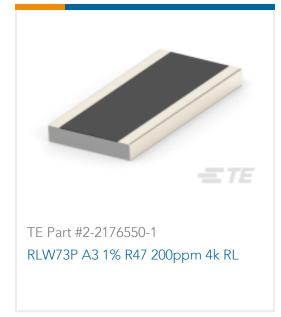
.056  $\Omega$ , Thick Film, Current Sensing Resistor, 1 %, 2 Termination, 1225, Taped & Reeled, 3 W, ±200 ppm/°C, Solder, Height .024 in [.6 mm], CGS RLW73
