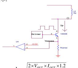
$$I_{P} = \sqrt{\frac{2 \times V_{OUT} \times I_{OUT} \times 1.2}{\eta \times L_{M} \times F \times K_{RF}}}$$
