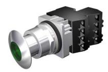
30mm Command/52, Chrome Finish Heavy Duty,Watertight/Oiltight Complete Metal Unit Illuminated Push-Pull Operator Full Voltage, 24V AC/DC LED Lamp Mushroom Head Cap Small 1 3/4" (44.5 mm) Metal, Chrome with Green Lens 3 Position Pull-Momentary/Push-Maintained 1 N.C.+1 N.C. Extra Late Break Heavy Duty Contacts, A600/P600 UL Listed, CSA Certified NEMA 1,3,3R,4,4X,12,13 & Automotive Standards
